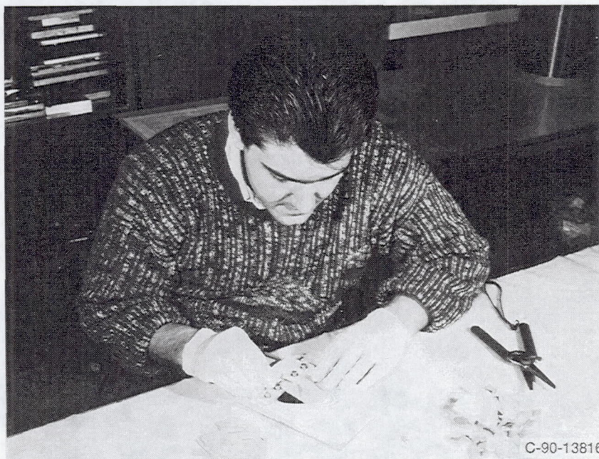
Figure 16.—Ply stacking fixture being used to stack CM-2D blade plies.
