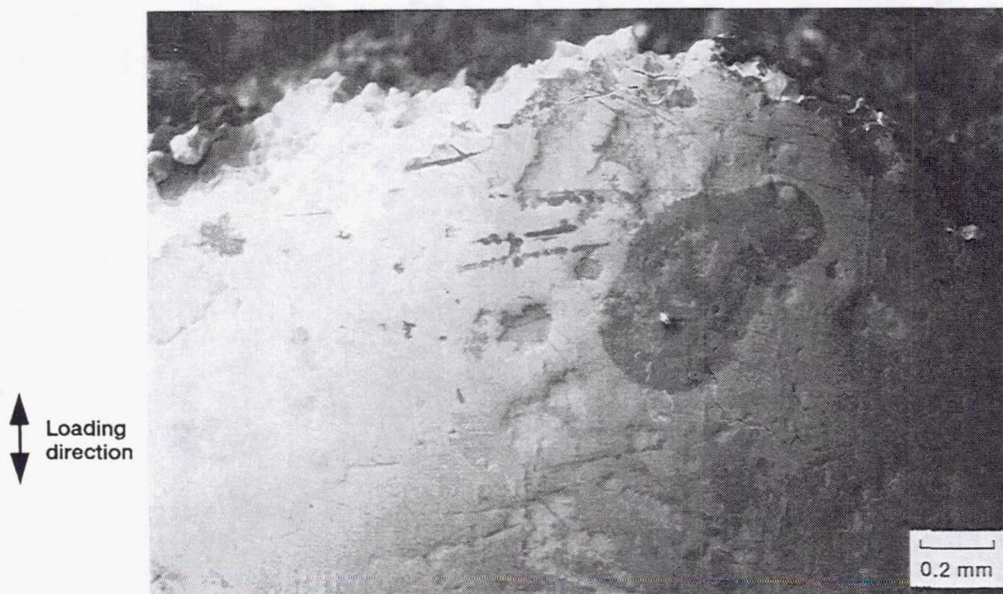
Figure 36.—SEM photomicrograph of the gauge surface of C+E NiAl specimen tested at 1000 K illustrating very limited damage ( \Delta\epsilon_p = 0.10 percent; N_f = 48\,090 ).
