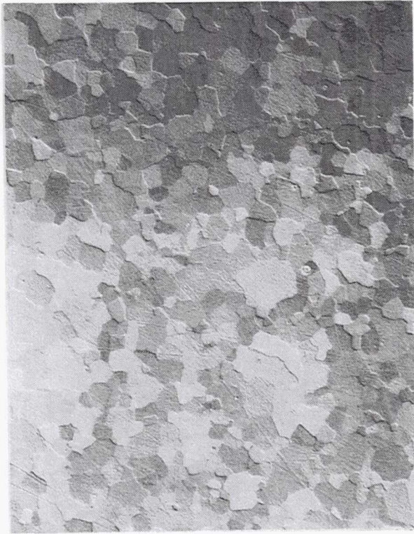
(a) As-received grain size is 18 \mu\text{m} .
