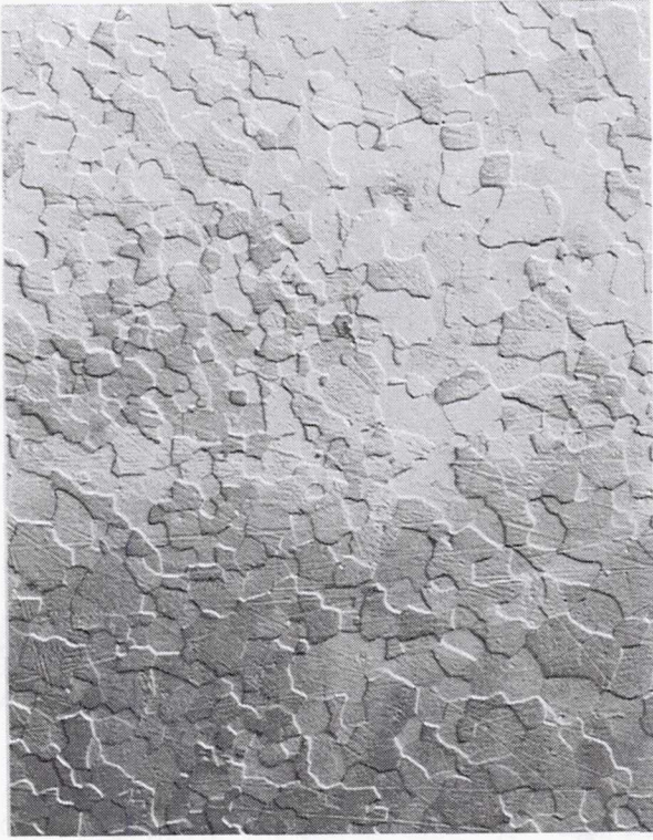
(b) Grain size is 18 \mu\text{m} after 80 h at 1000 K.
