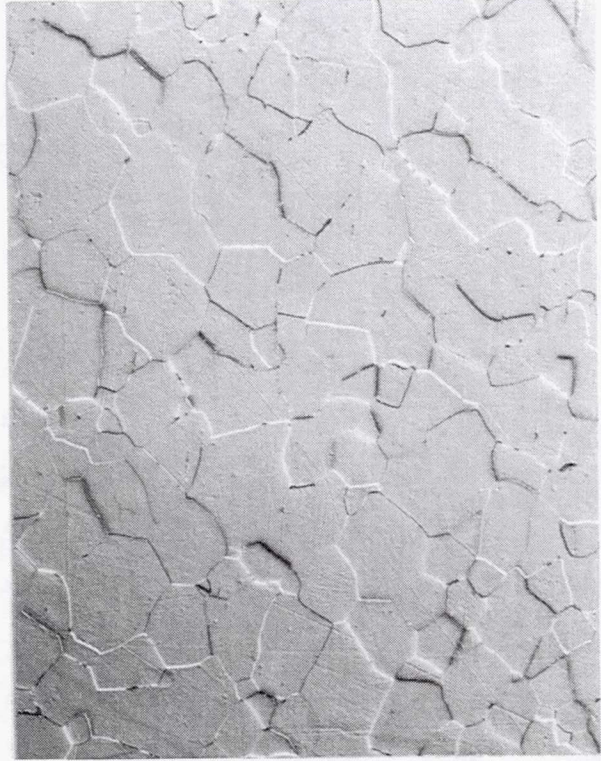
(c) Grain size is 75 \mu\text{m} after fatigue testing at 1000 K.
