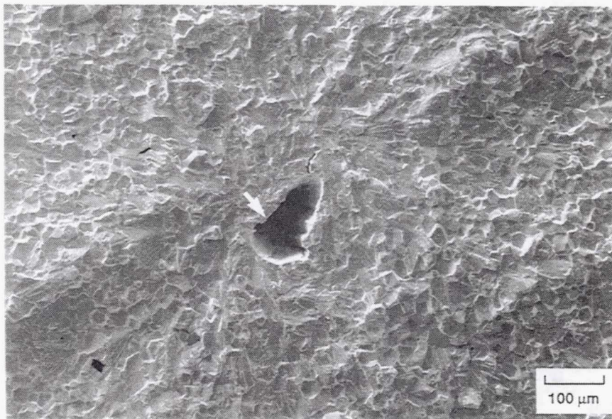
Figure 9.—Fractograph showing large teardrop shaped void (arrow) at crack initiation site in C+E specimen tested at 300 K ( \Delta\epsilon_p = 0.10 percent; N_f = 269 ).
