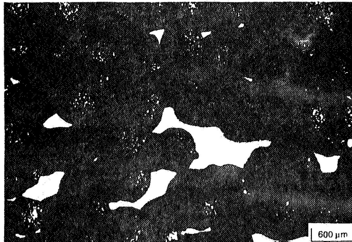
SINTERED UC 2 MICROSPHERES
