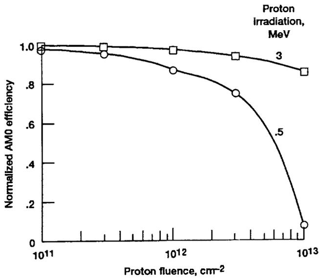
Figure 3.—Changes in AMO conversion efficiency of heteroepitaxial InP solar cells with fluence for 0.5- and 3-MeV proton irradiations.
