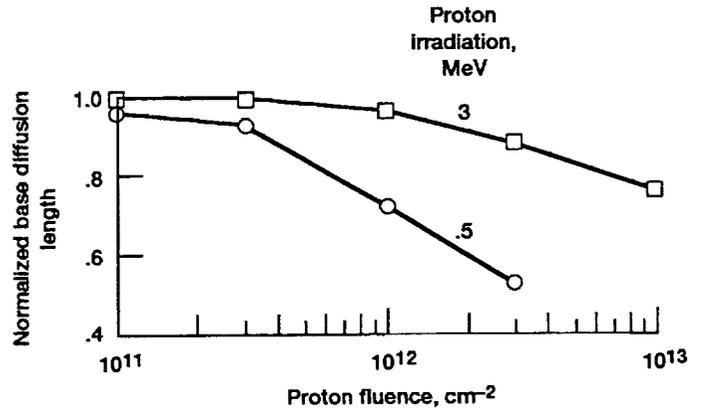
Figure 4.—Variation of base diffusion length with fluence in heteroepitaxial InP solar cells after 0.5- and 3-MeV proton irradiations.
