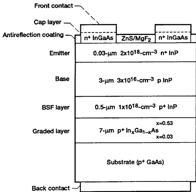
Figure 1.—Structure of metalorganic, chemical-vapor-deposited n<sup>+</sup> pp<sup>+</sup> InP/In<sub>x</sub>Ga<sub>1-x</sub>As/GaAs solar cell.
