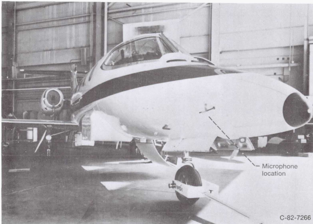
Figure 8.—Learjet nose microphone installation.
