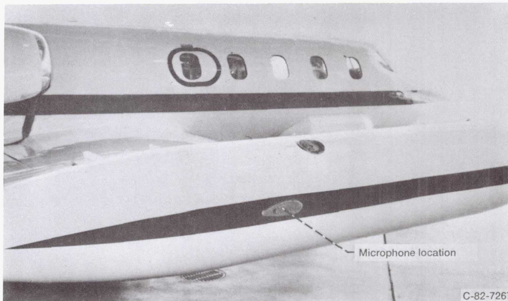
Figure 6.—Learjet wingtip microphone installation.
