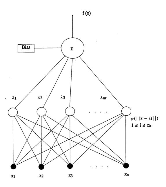
Figure 1: Single linear output radial basis function network
