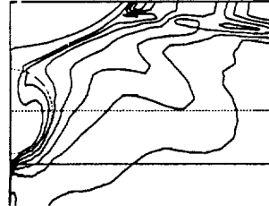
4. Axial velocity contours at the propeller plane X/L = 0.976 ( U/U_\infty = 0.3, 0.4, 0.5, 0.6, 0.7, 0.8, 0.9 )
