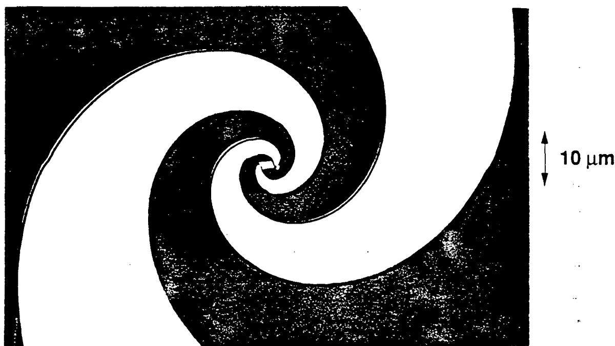
Figure 1. Photograph of the antenna-coupled microbolometer
