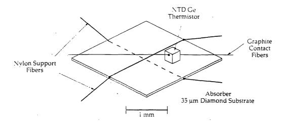
Figure 2: Sketch of a composite bolometer
