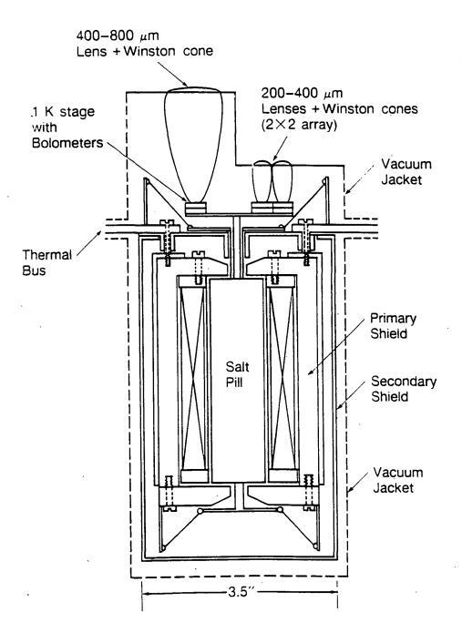
Figure 1: Adiabatic demagnetization refrigerator
