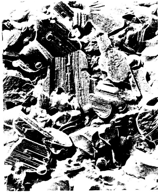
Figure 5. Replica electron micrograph of the fracture surface of enstatite- \beta -spodumene-zirconia glass-ceramic E-1. Twinning in the enstatite is seen to influence the fracture path; spodumene grains are smooth.
