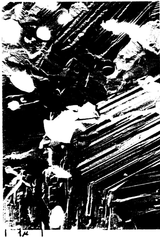
Figure 6. Fracture surface (REM) of enstatite-zircon glass-ceramic E-2 showing interlocking twinned enstatite grains and nodular zircon. Note the step splintering effect of the intersection of cleavage and twinning.
