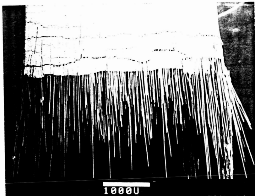
Figure 9. Non-brittle fracture mode of Nicalon®/glass-ceramic matrix composites.
