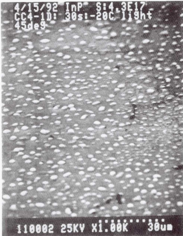
Figure 11.—n-InP: S:4.3E17 etched .5 min.
