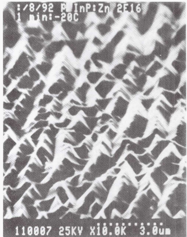
Figure 6.—p-InP: Zn:2E16 etched 1 min.
