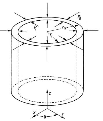
Figure 6. Stresses in a Cylinder Wall
