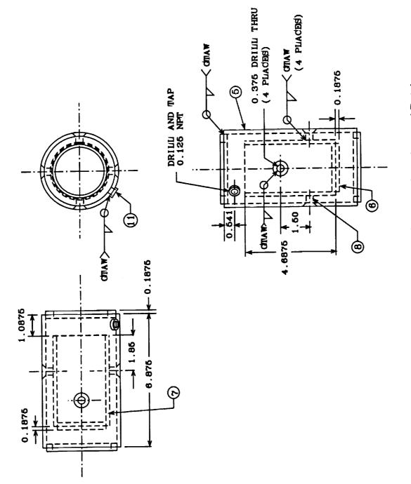
Figure 47. Detailed Drawing of the Cartridge Container and Retainer
