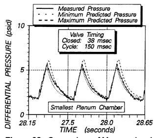
Figure 32. Comparison of Measured and Predicted Plenum Chamber Pressure During Test Number 8
