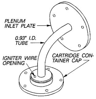
Figure 3. Container Cap and Plenum Inlet Plate Subassembly
