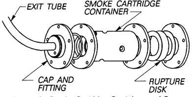
Figure 2. Smoke Cartridge Container and Cap
