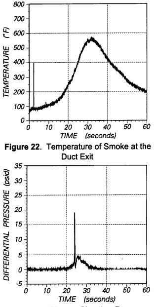
Figure 23. Plenum Chamber Pressure Differential with Smoke Flow Diverted
