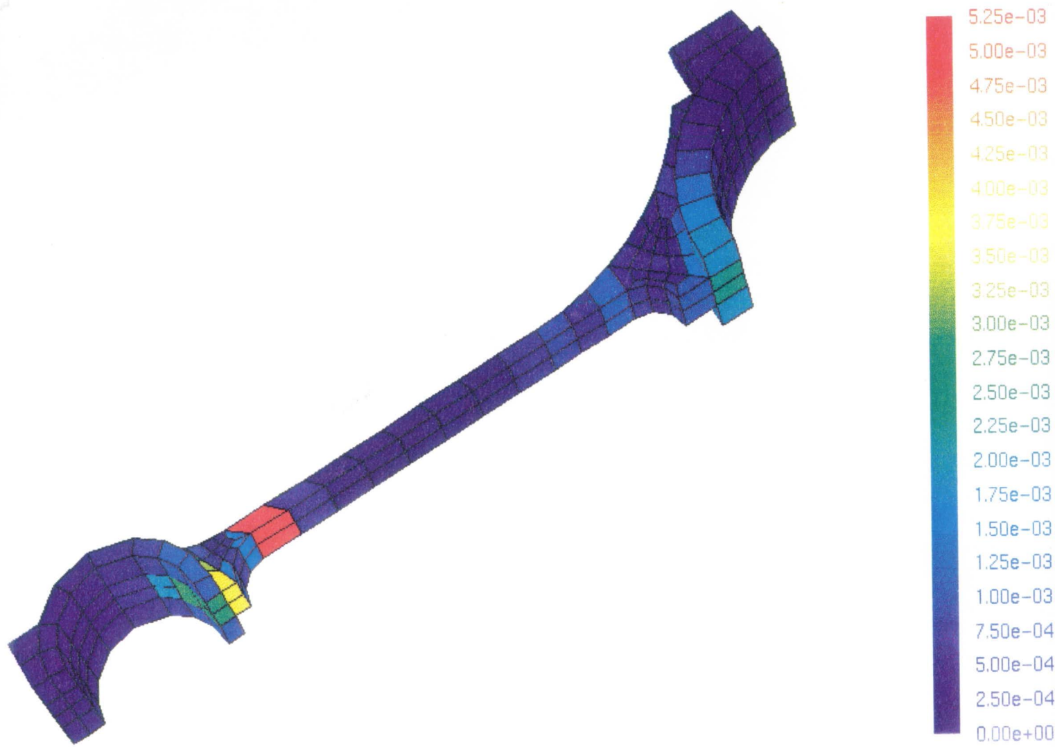
Figure 5.11: Residual error estimation distribution for a steady state solution of a three-dimensional connecting rod
