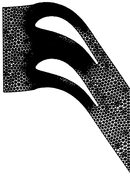
Figure 6.22 Sanz subcritical turbine cascade 1 st adapted mesh: 1,018 nodes and 1,799 elements.
