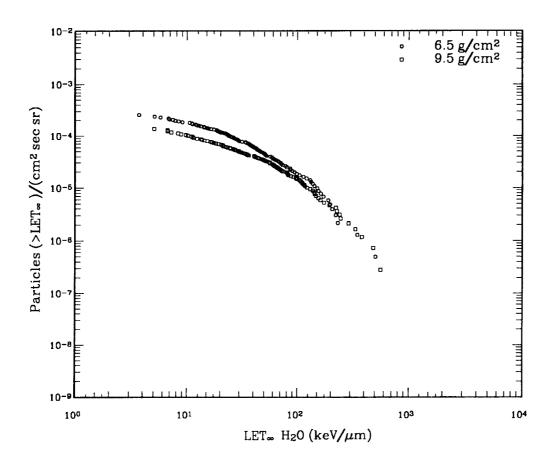
Figure 2: LET Spectra measured in the main stack beneath two shielding depths. Curve  $\circ$  was under 6.5 g/cm<sup>2</sup> and Curve  $\square$  was under 9.5 g/cm<sup>2</sup>. Both spectra were measured in CR-39/DOP using the track coincidence method.
