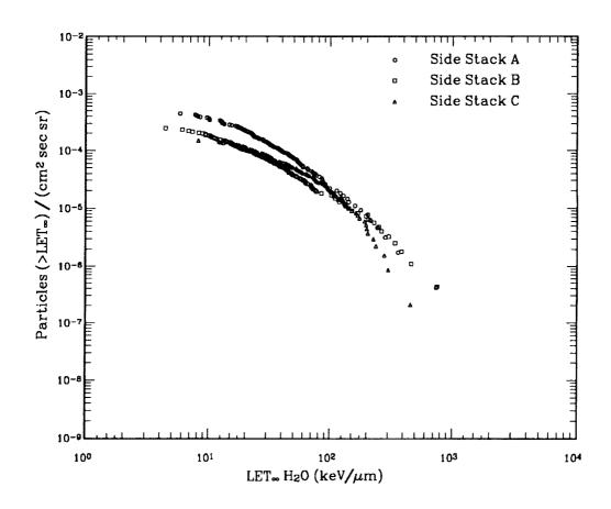
Figure 3: LET Spectra in side stacks showing effect of orientation of detectors. Curve  $\circ$  is from side stack A and faced toward space/north. Curve  $\square$  is from side stack B and faced Earth/north. Curve  $\triangle$  is from side stack C and faced Earth/south. All three spectra were measured in CR-39/DOP under a shielding of 1.3 g/cm<sup>2</sup>.
