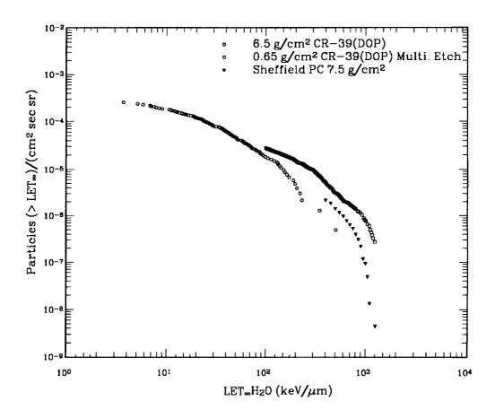
Figure 4: Measurements of the high LET tail in PC and CR-39(DOP).
