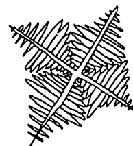
SCHEMATIC SHOWING THE APPEARANCE OF THE SOLID-LIQUID INTERFACE FOR AN ISOLATED EQUIAXED DENDRITE GROWING IN A LIQUID METAL
