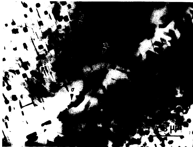
Figure 12. PFZ in sample A11M after 26 hours at 200°C.
