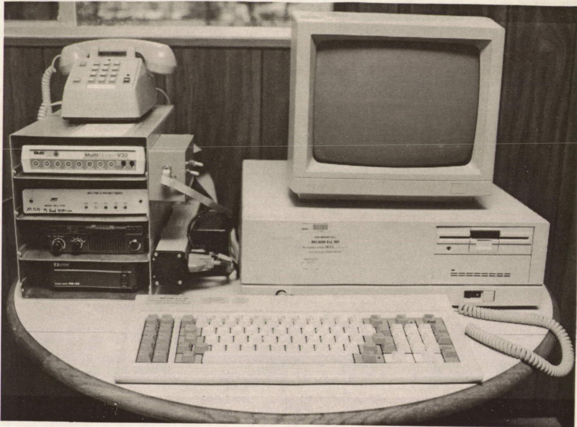
Figure 3 - TDWR Data Link Ground Station
