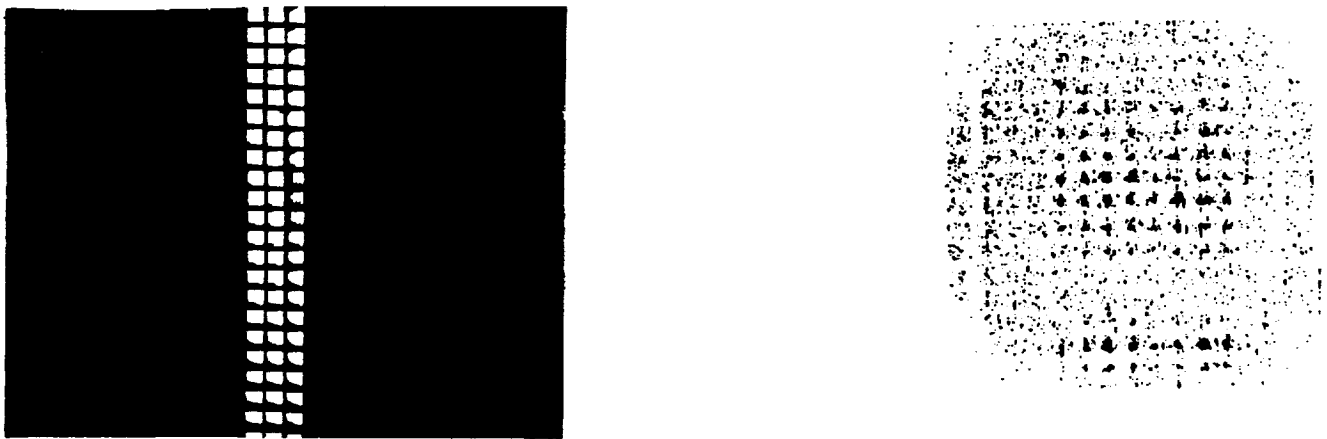
Figure 2 – 3: a: Photograph showing 3 x 16 pore region of square channel MCP b: X-ray image of point source through aperture.
