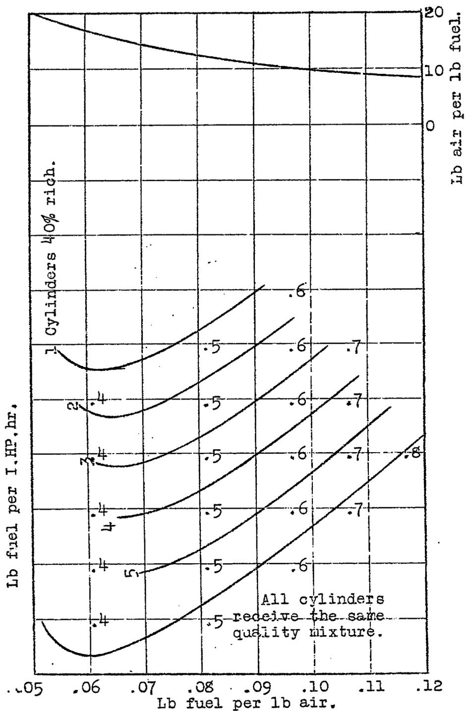
Fig.11. Effect of changes in distribution - 6 cylinder engine.
