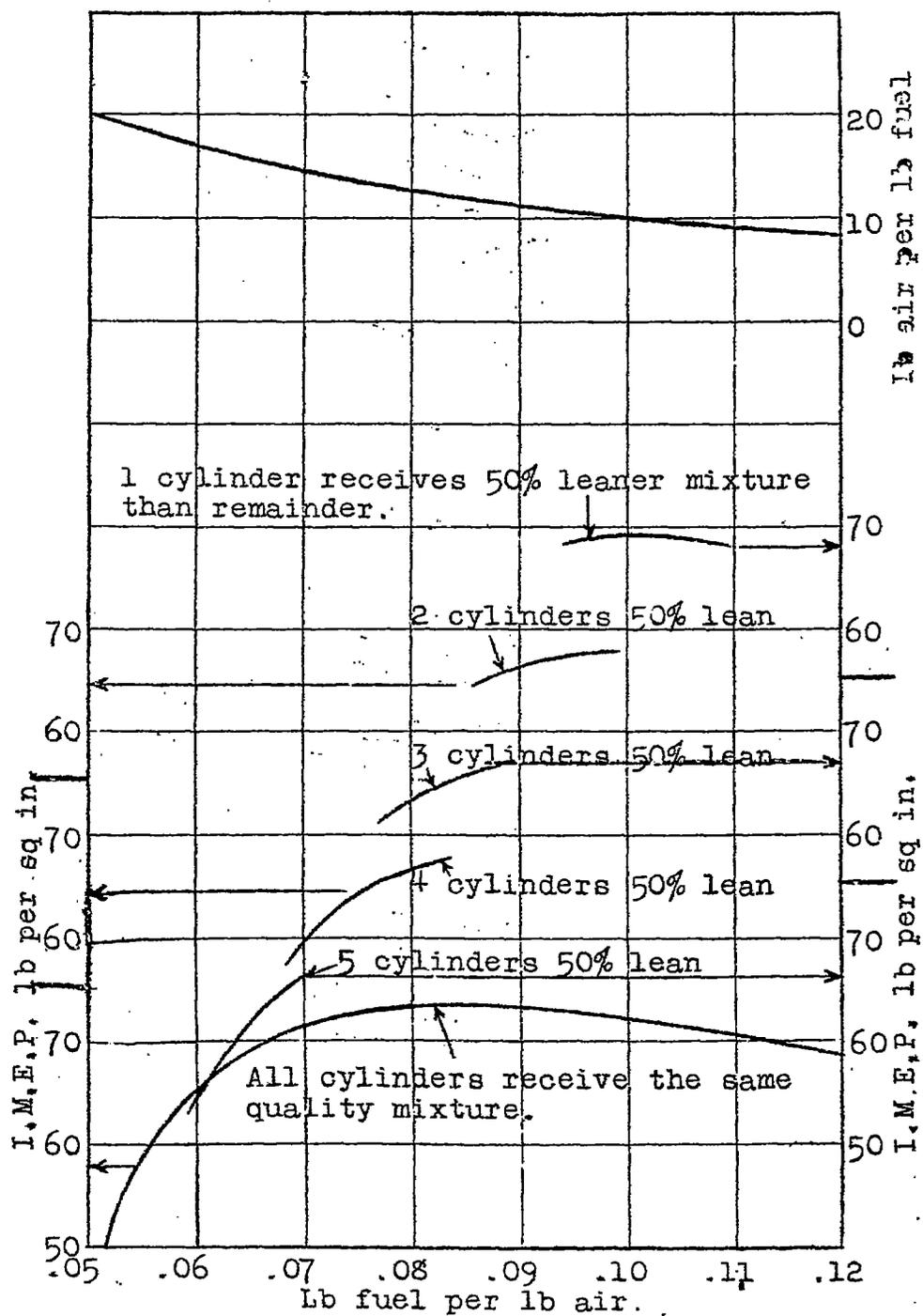
Fig.6. Effect of changes in distribution - 6 cylinder engine.
