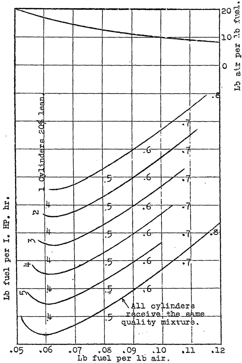
Fig.3. Effect of changes in distribution-6 cylinder engine.
