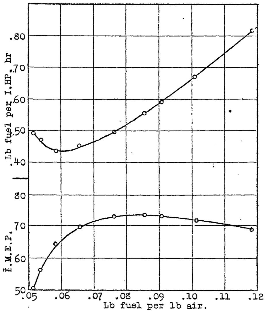
Fig.1. Single cylinder engine test.
