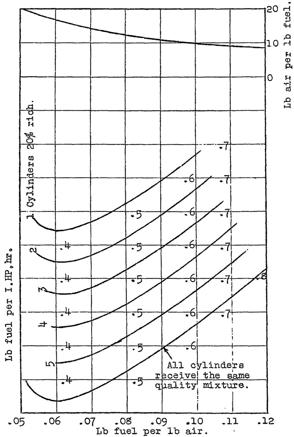
Fig.9. Effect of changes in distribution - 6 cylinder engine.
