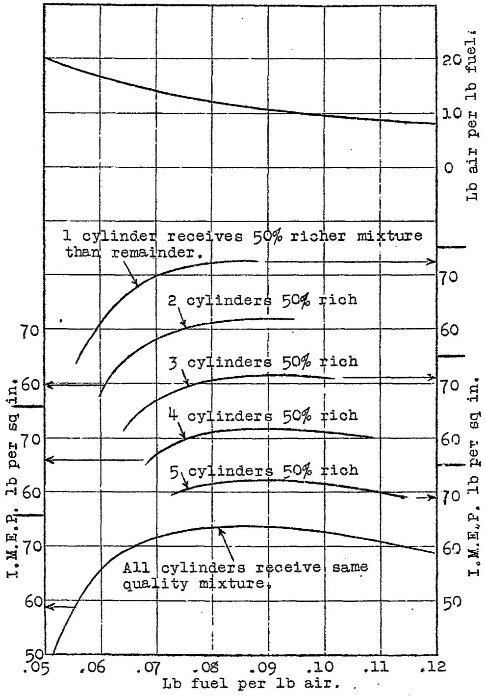
Fig.12. Effect of changes in distribution - 6 cylinder engine.
