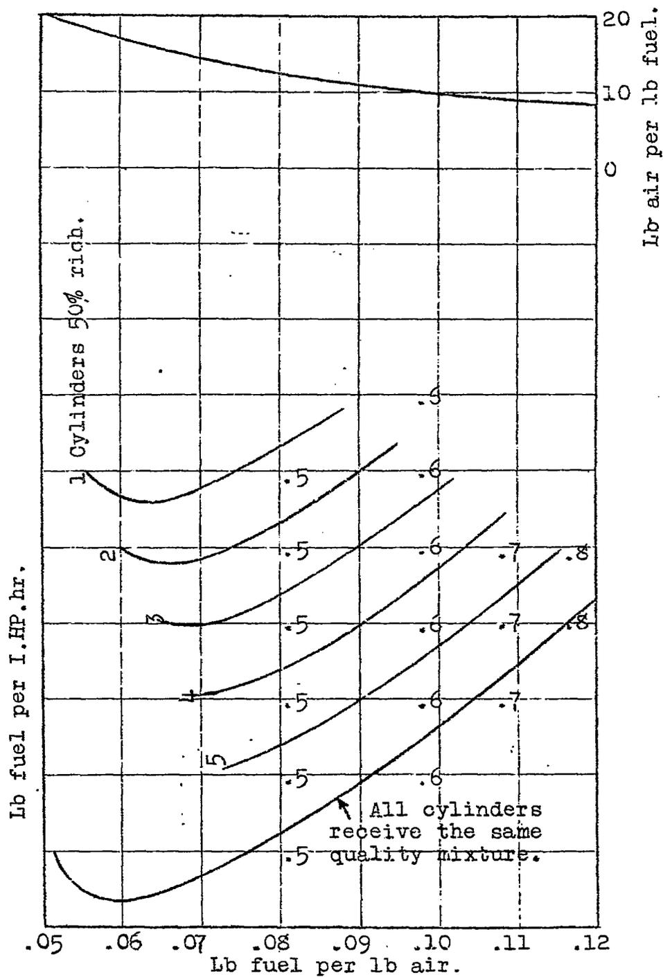
Fig.13. Effect of changes in distribution - 6 cylinder engine.
