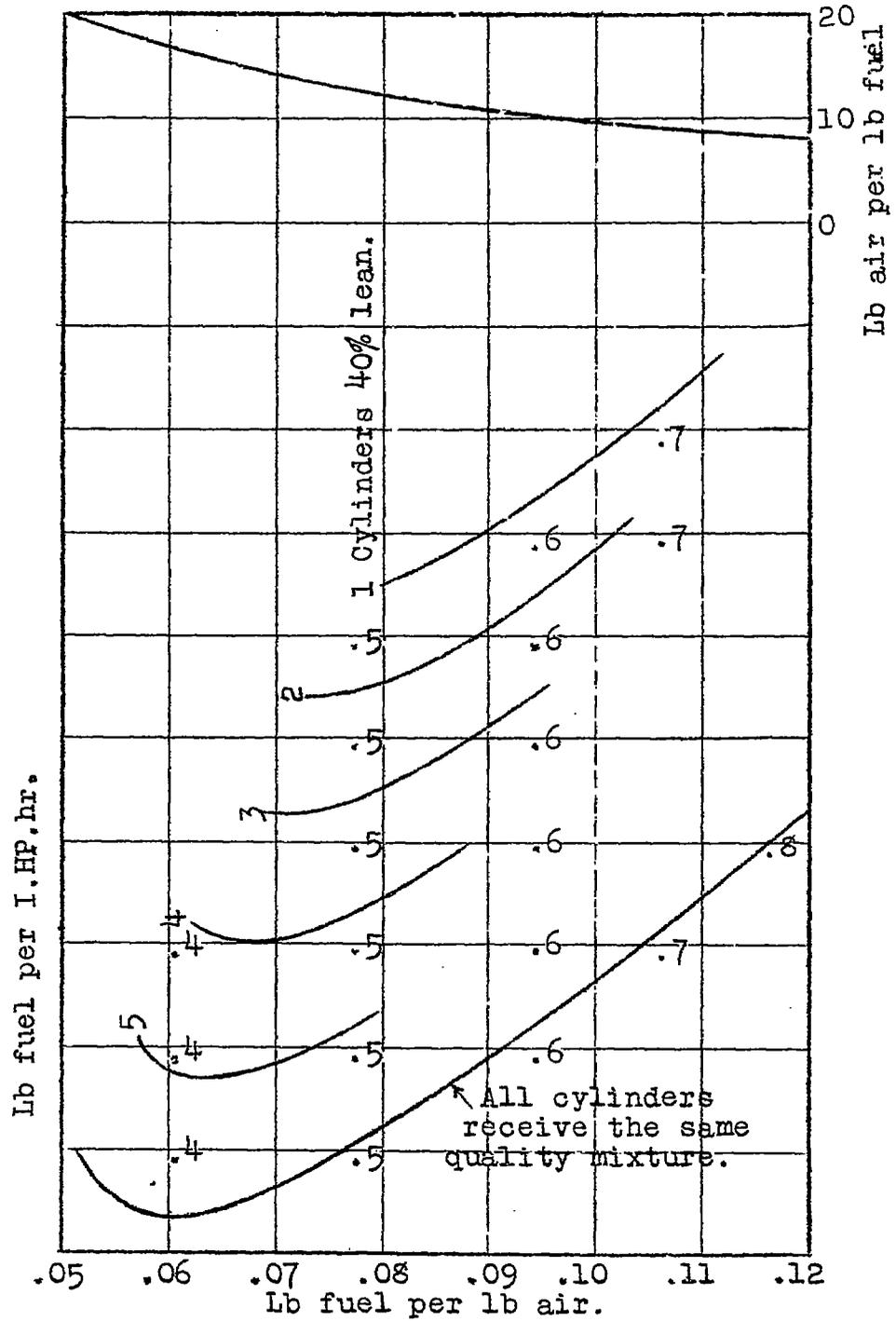
Fig. 5. Effect of changes in distribution - 6 cylinder engine.
