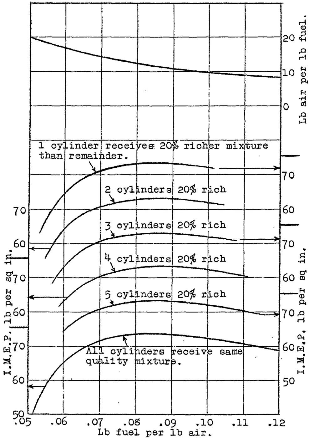
Fig. 8. Effect of changes in distribution - 6 cylinder engine.
