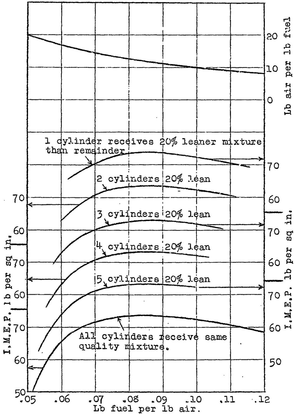
Fig.2. Effect of changes in distribution-6 cylinder engine.
