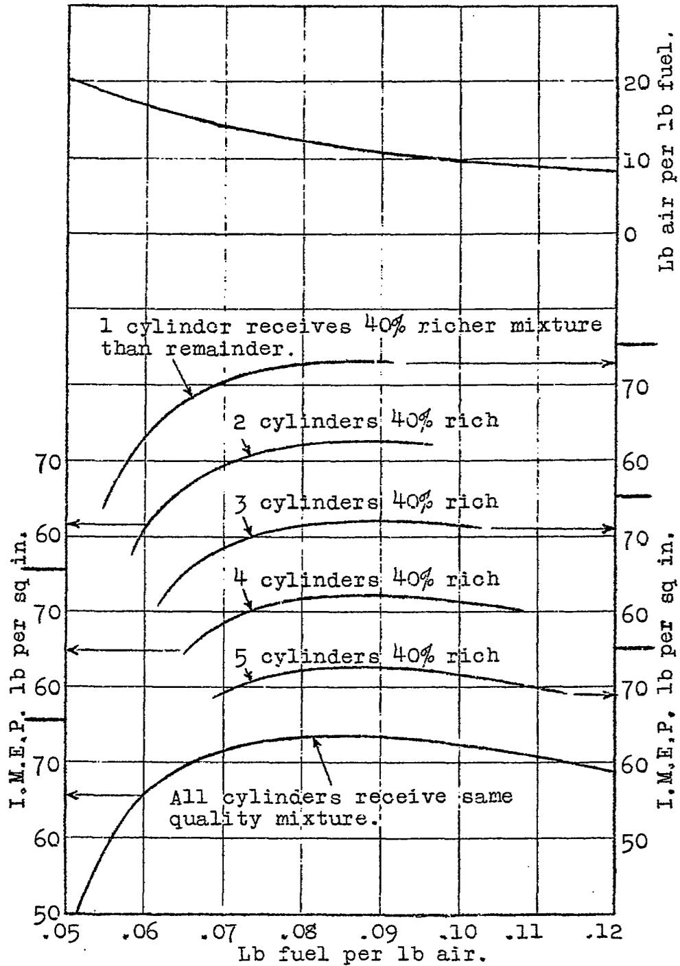
Fig.10. Effect of changes in distribution - 6 cylinder engine.
