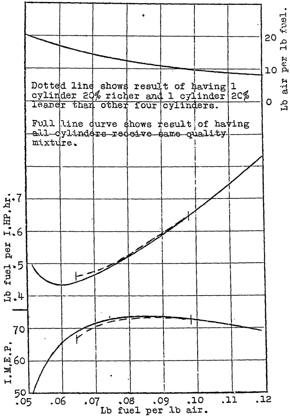
Fig.14. Effect of changes in distribution - 6 cylinder engine.
