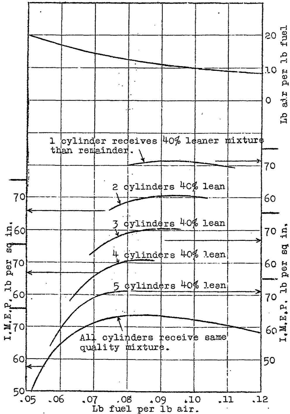
Fig.4. Effect of changes in distribution - 6 cylinder engine.
