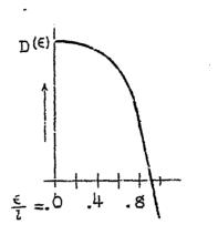
with elliptical distribution of lift on the lower wing,  $D(\epsilon)$  is negative at the ends of the upper wing, that is, the acceleration is here directed upward, so that the actual angle of attack of the upper wing becomes larger at the ends. The turning up of the wing tips, therefore, appears justifiable.
