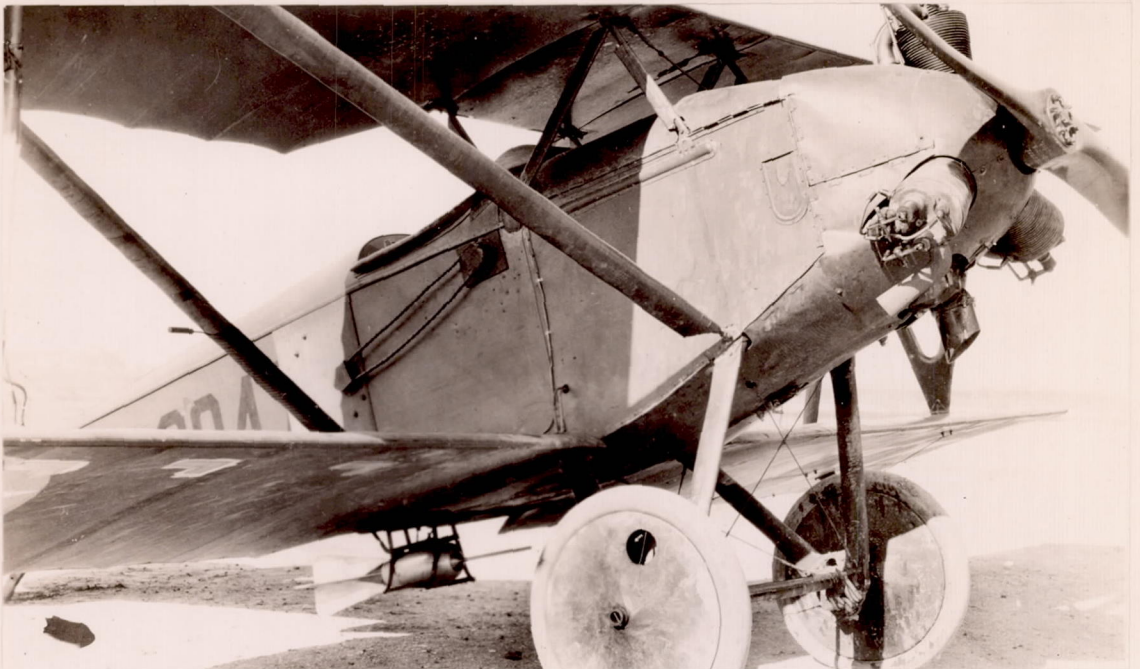
Fig.11 Flight-path-angle and air-speed recorder mounted in cradle, ready for taking off and landing.
