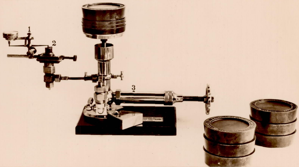
Fig. 3 Diaphragm test apparatus using Ashton dead-weight gauge tester 1. L.S.Starrett dial test indicator. 2. Injection valve holding diaphragms under test. 3. Ashton dead weight gauge tester.
