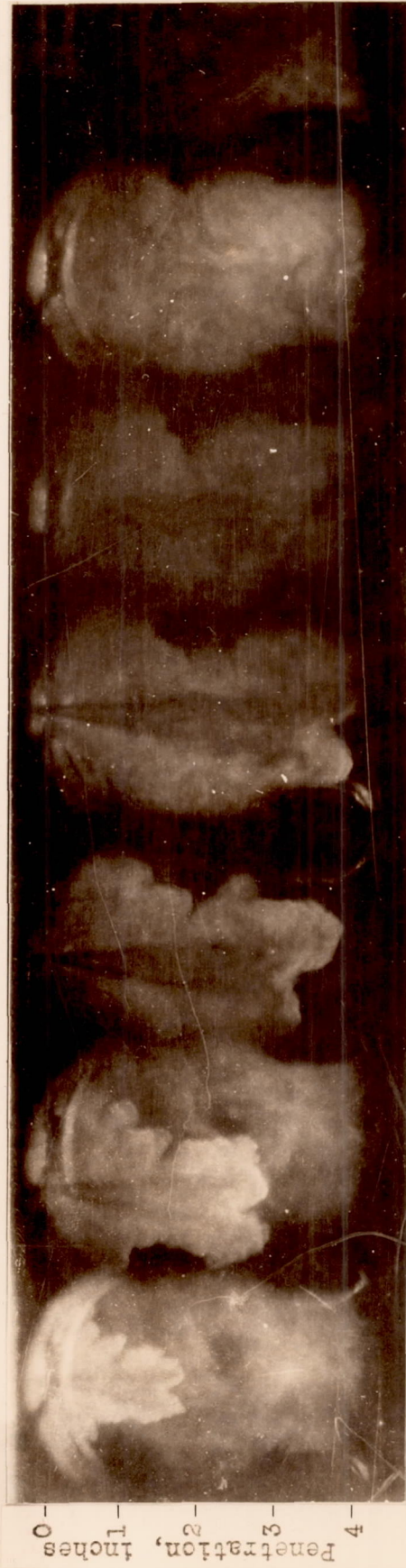
Fig. 21 Nozzle No. 9, injection pressure 4750 lb. per sq. in.
