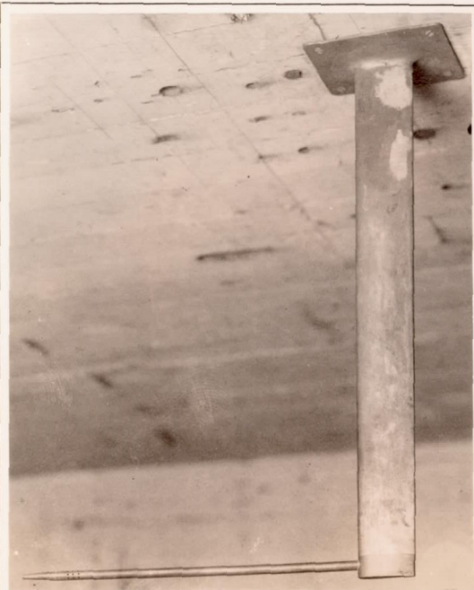
Fig.1 Pitot- static tube in work- ing part of 6 - foot tunnel
