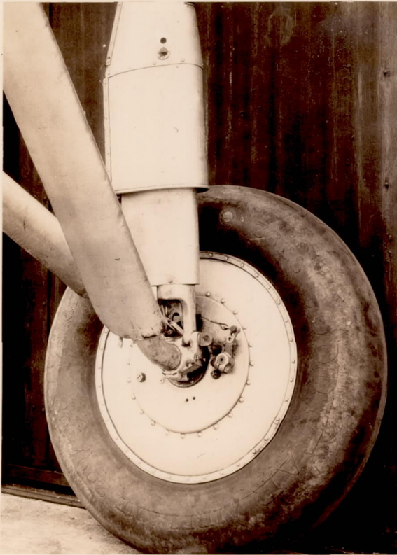
Fig.1 The wheel brake as applied to the Douglas M3 for the landing run tests.
