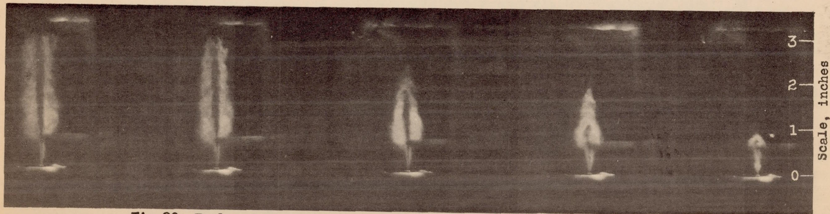
Fig.20 Fuel and air jets intersecting at right angles. Air jet moving away from camera lens. Fuel-injection pressure, 500 pounds per square inch. Air-jet injection pressure, 500 pounds per square inch. Chamber-air density, 1.1 pounds per cubic foot.
