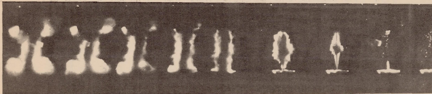
Fig. 15 Opposed sprays with the nozzles close together. Fuel-injection pressure, 4,000 pounds per square inch. Chamber-air density, 1.1 pounds per cubic foot. Distance between open nozzles, 1.5 inches.
