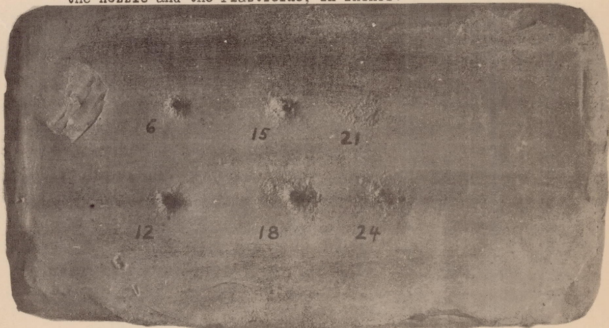
Fig.3 Impressions made in Plasticine by fuel sprays injected through air having a density of 0.076 pounds per cubic foot. Fuel-injection pressure - 4,000 pounds per square inch. Valve-opening pressure - 3,500 pounds per square inch. Figures beside each impression indicate the distance between the nozzle and the Plasticine, in inches.
