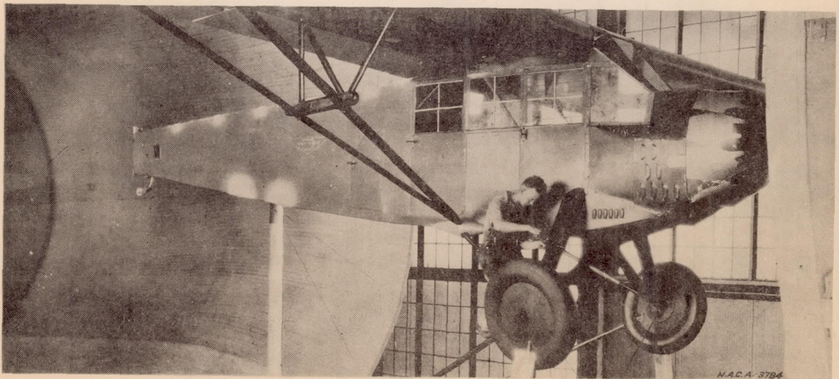
Fig. 5. ENGINE REMOVED AND NOSE FAIRED.
