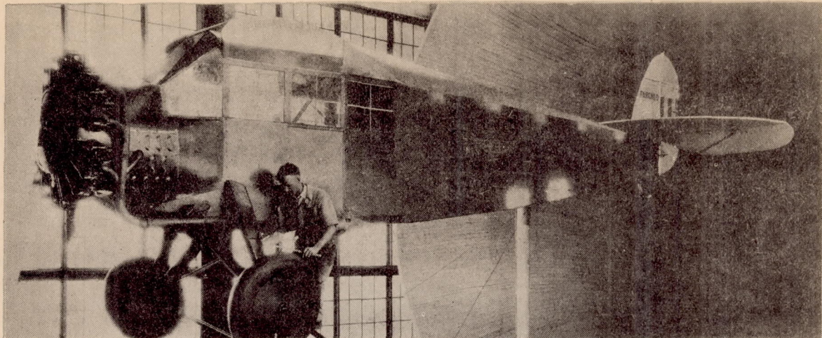
Fig. 9. TURTLEBACK AND WING ROOT FAIRINGS ADDED.
