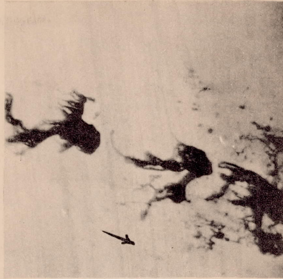
Injection pressure, 550 lb./sq.in. Orifice diameter, 0.020 inch Distance from nozzle, 5 inches
