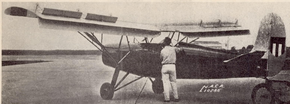
Figure 3.- Fairchild 22 airplane showing bal- anced split flap and re- tractable ailerons
