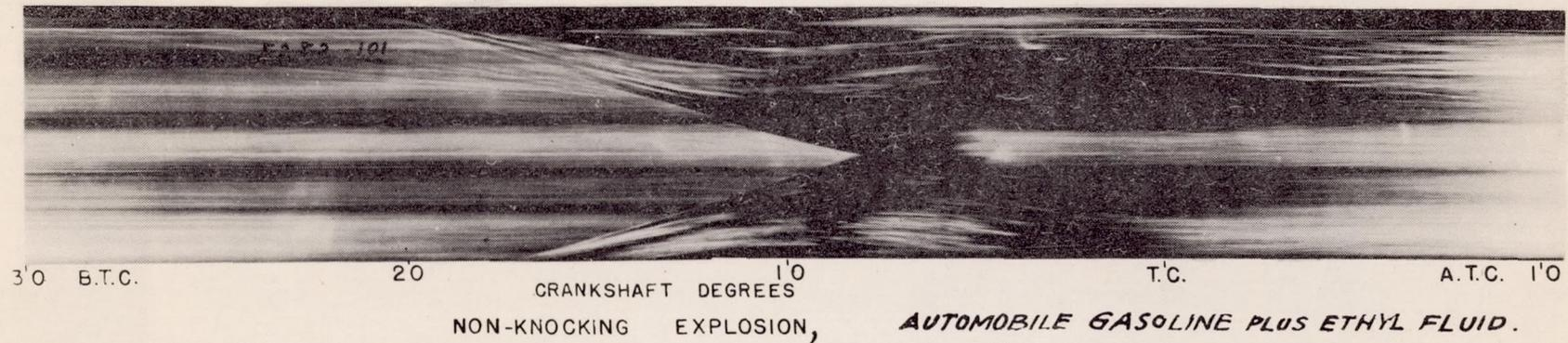
FIGURE 10. SCHLIEREN PHOTOGRAPHS SHOWING TWO FLAME FRONTS PASSING THROUGH EACH OTHER
