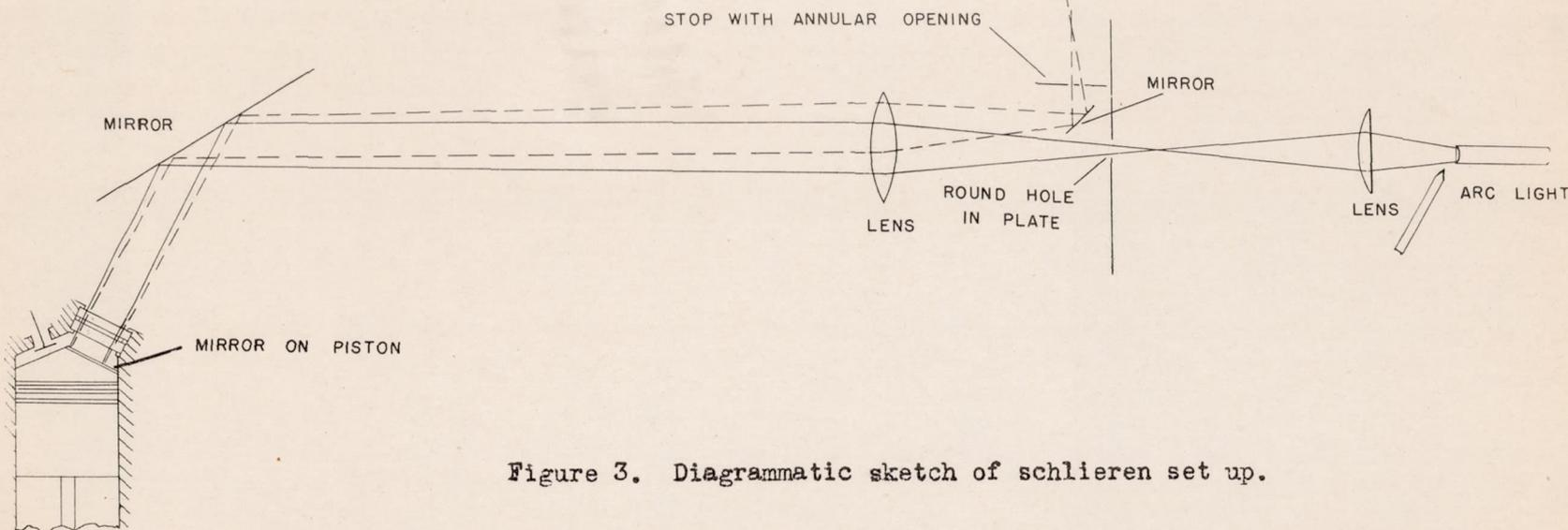
Figure 3. Diagrammatic sketch of schlieren set up.
