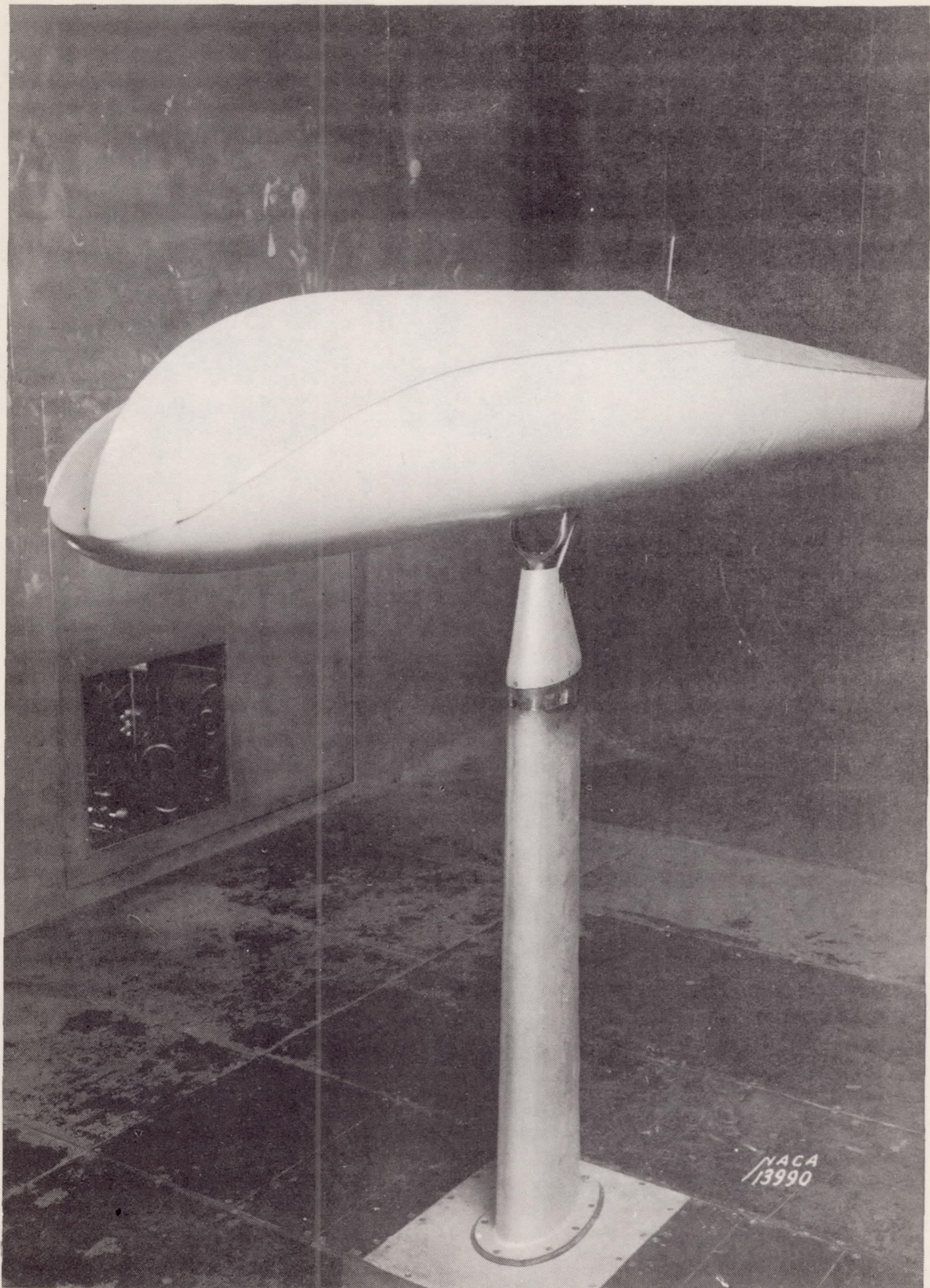
Figure 6.- Typical float installation in the 7- by 10- float wind tunnel. ( Model shown not reported)
