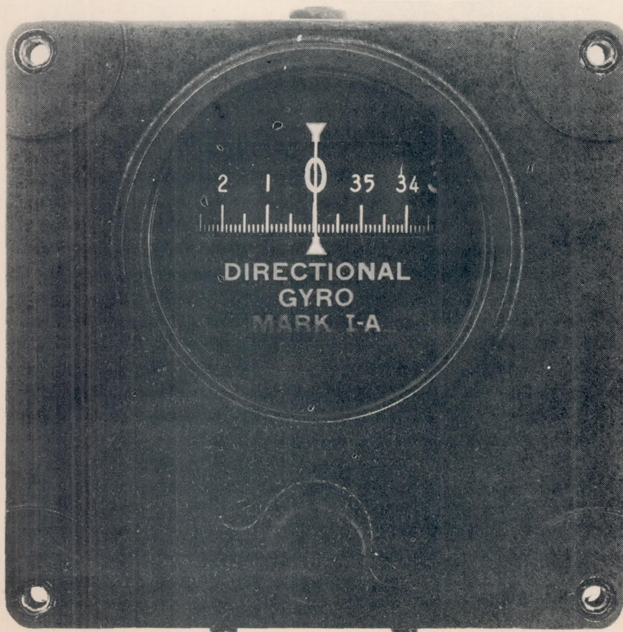
Figure 5.- Photograph of Sperry direction- al gyro.
