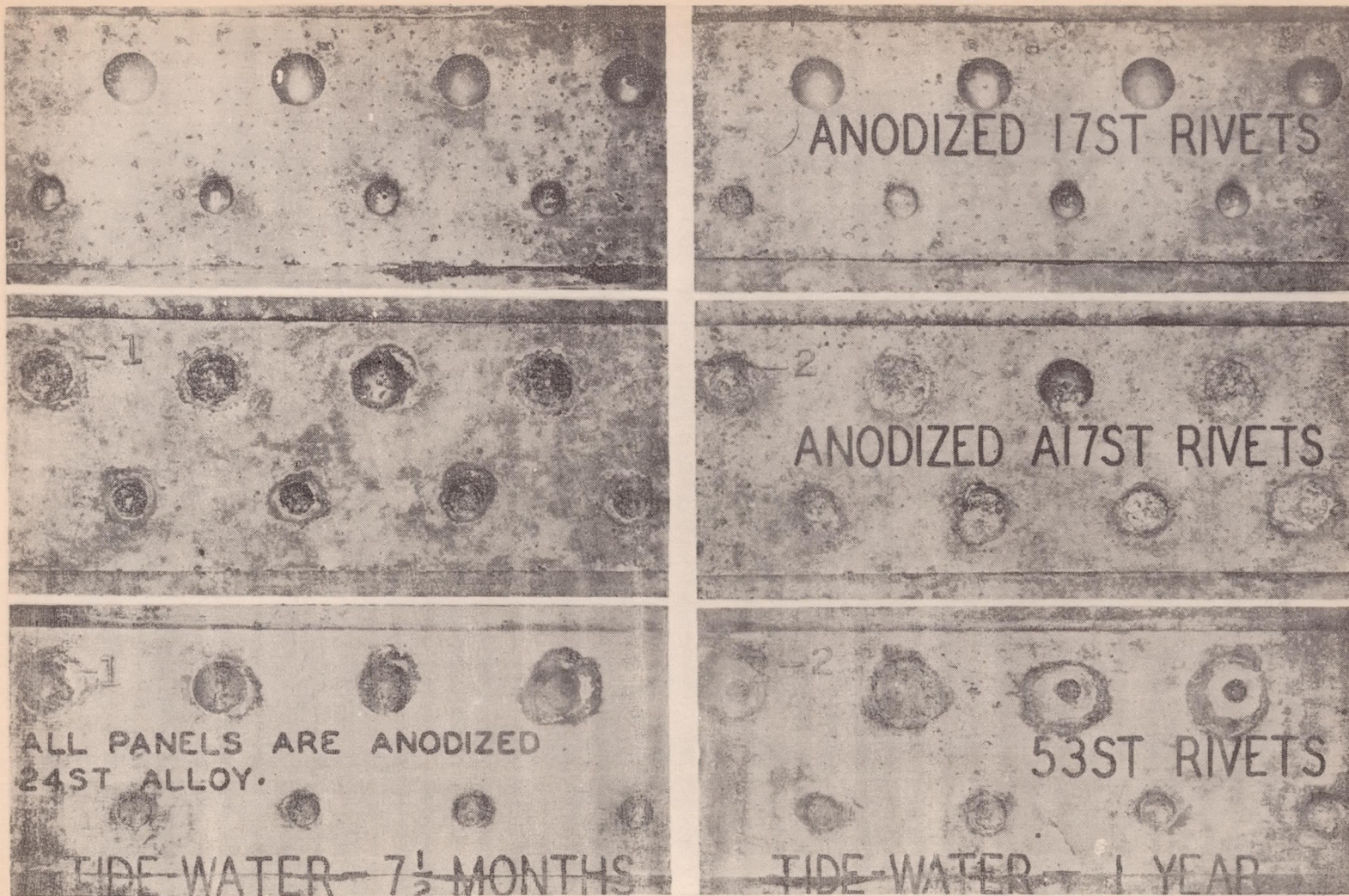
Figure 4.- Rivets used on anodized 24ST alloy panels exposed to tidewater. Note the severe corrosion on anodized A17ST and 53ST rivets, and the relatively slight attack on anodized 17ST rivets. In this, and all of photographs which follow, the large letters at the right apply to the entire horizontal rows, while those at the tops or bottoms apply to the entire vertical rows. \times 1
