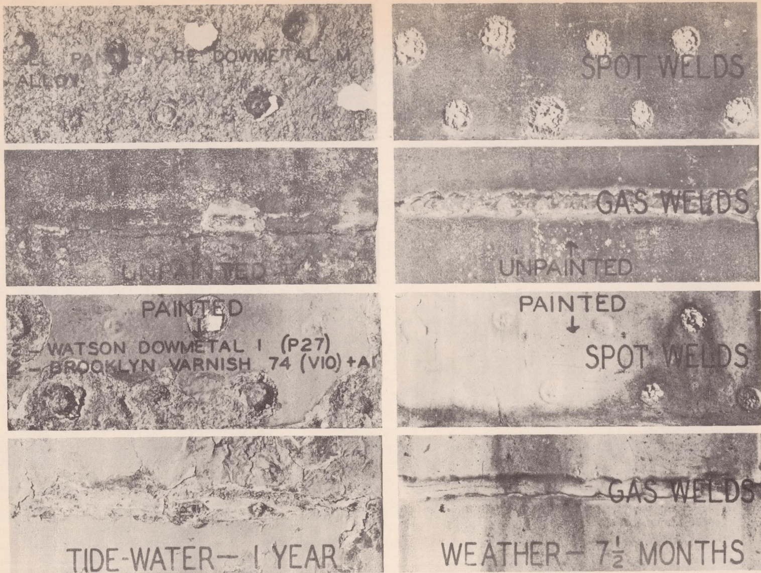
Figure 12.- Welded Dowmetal M alloy panels exposed to tidewater or to the weather. The spot welds were very susceptible to attack, but the gas welds were quite resistant. \times 1
