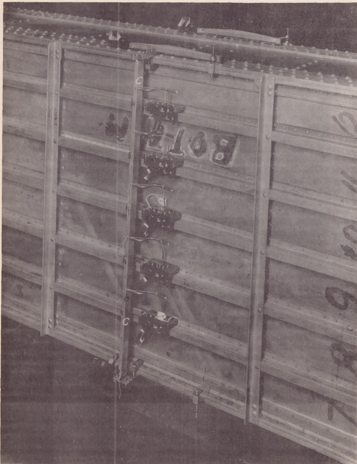
Figure 7- Mounting of strain gages on stringers and corner posts.
