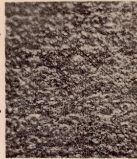
Figure 3.- Photo- micro- graph of polished surface of wing (10X)
