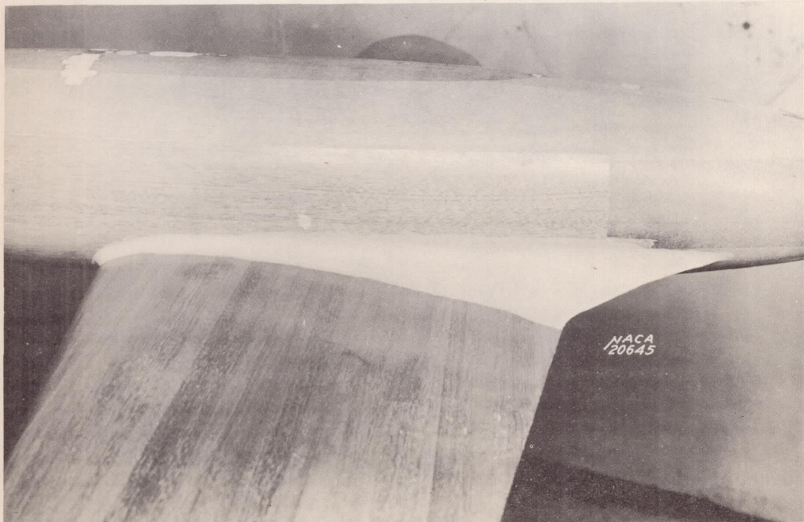
Figure 2b.- Side view of wing fillet on low-wing monoplane model tested in the NACA 7- by 10- foot wind tunnel.
