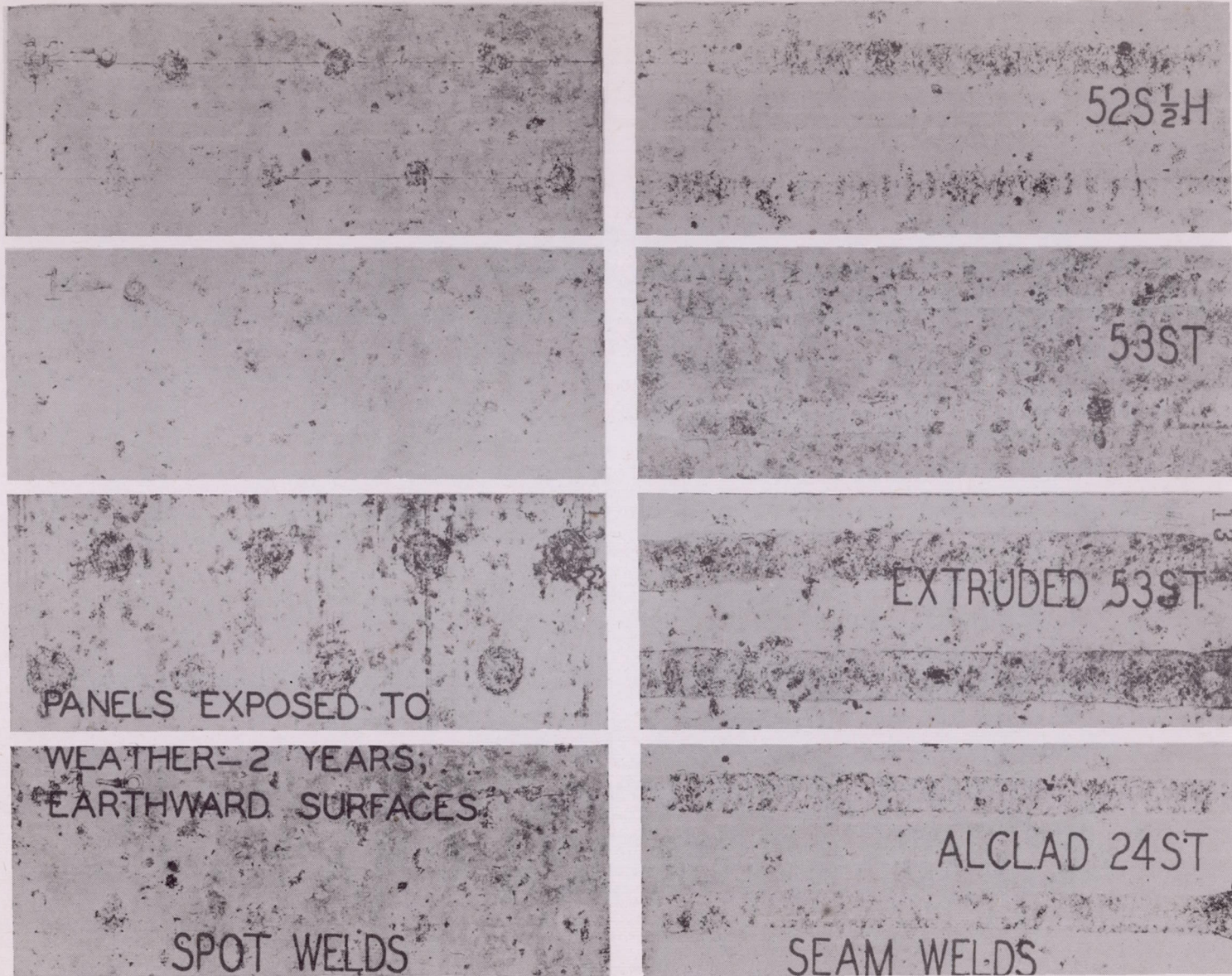
Figure 11.- Welded aluminum-alloy panels exposed to the weather were more corroded than those exposed to tidewater, especially at the welds. x 1 (11).
