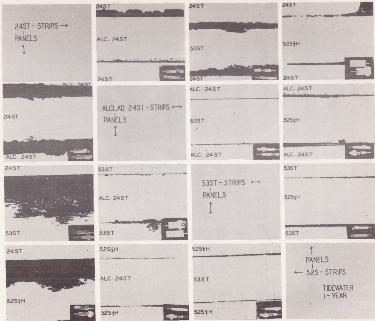
Figure 15.- Cross sections showing aluminum alloys exposed to tidewater in contact with each other. Note that the Al-clad 24ST, 52S-1/2H, and 53ST were anodic to 24ST alloy and were especially severely attacked when 24ST was the main panel. The lack of proximity of strips to the panels, in some instances, is a criterion of the amount of accumulated corrosion products at the faying surfaces which forced the sheets to separate. Photomicrographs, x 25; smaller cross section, x 1/2. (13 and 14).
