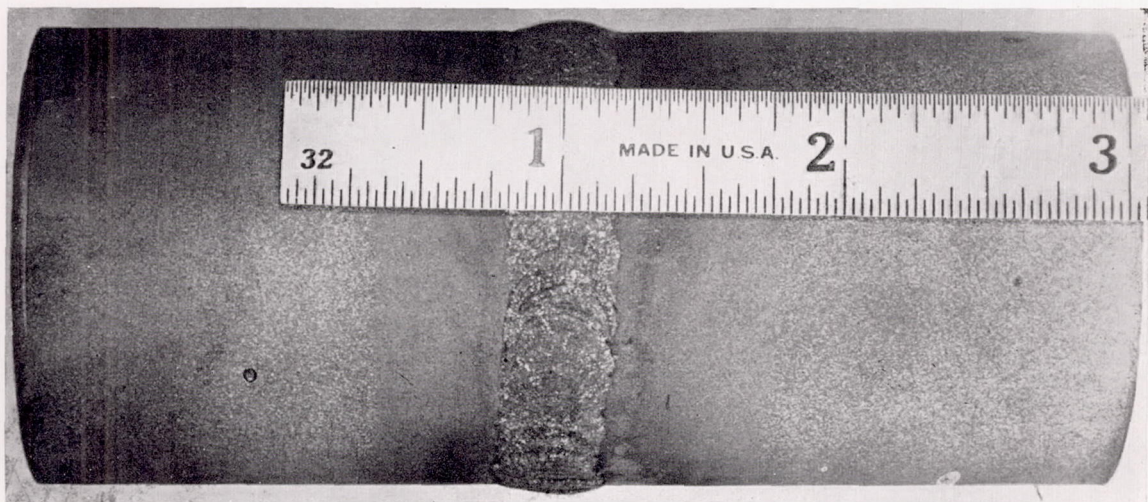
FIGURE 49.—Macrostructure of the weld and adjacent material, showing the various heat-affected zones.
