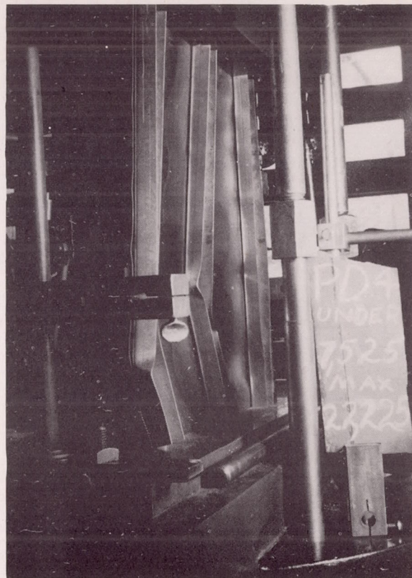
Figure 31.- Panel PD-4 under 7,525 pounds after subjection to 22,225 pounds.
