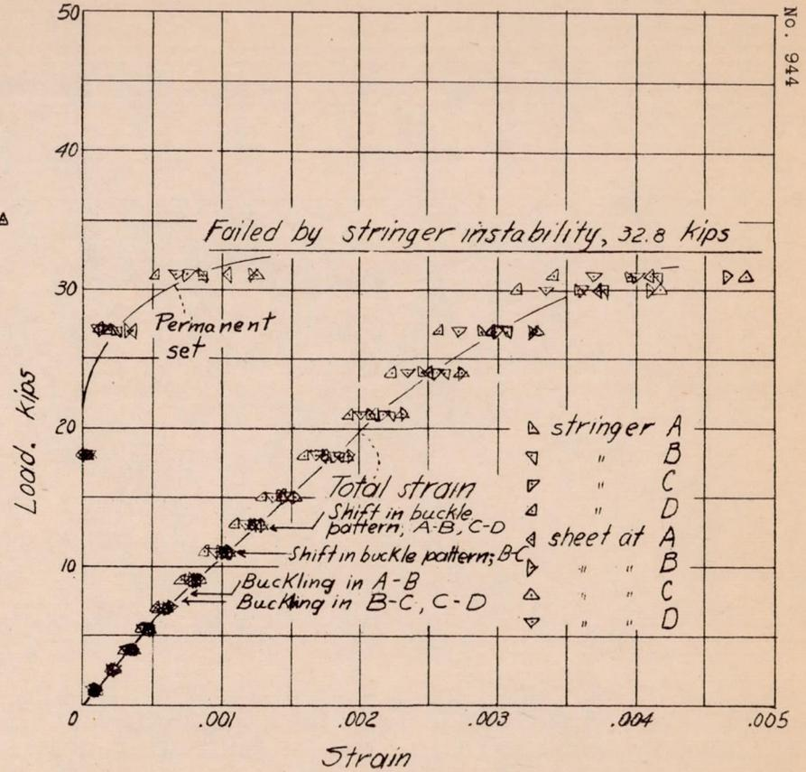
Figure 7.- Test of panel 2; radius, 38.2 inches.
