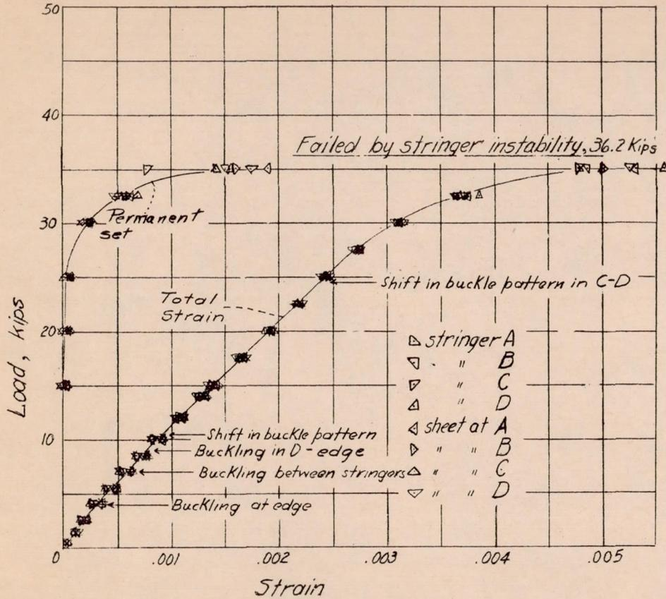
Figure 6.- Test of panel 1; radius, 76.5 inches.
