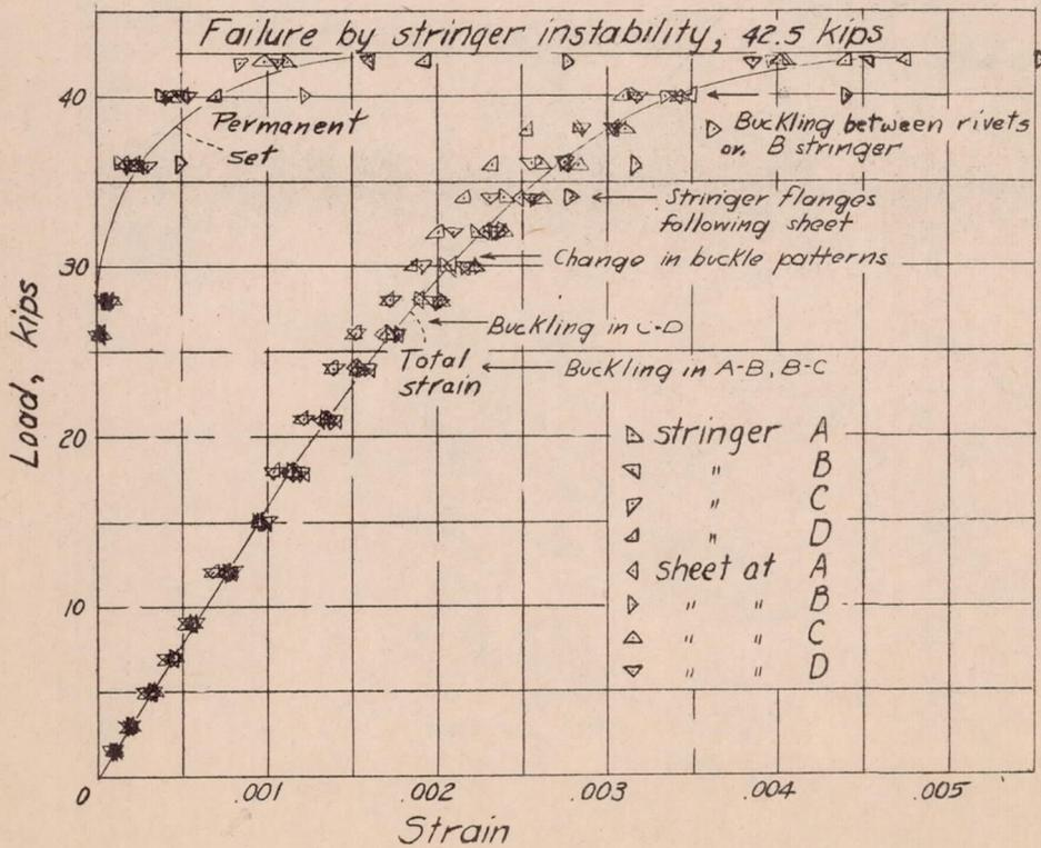
Figure 15.- Test of panel 10; radius, 25.5 inches.
