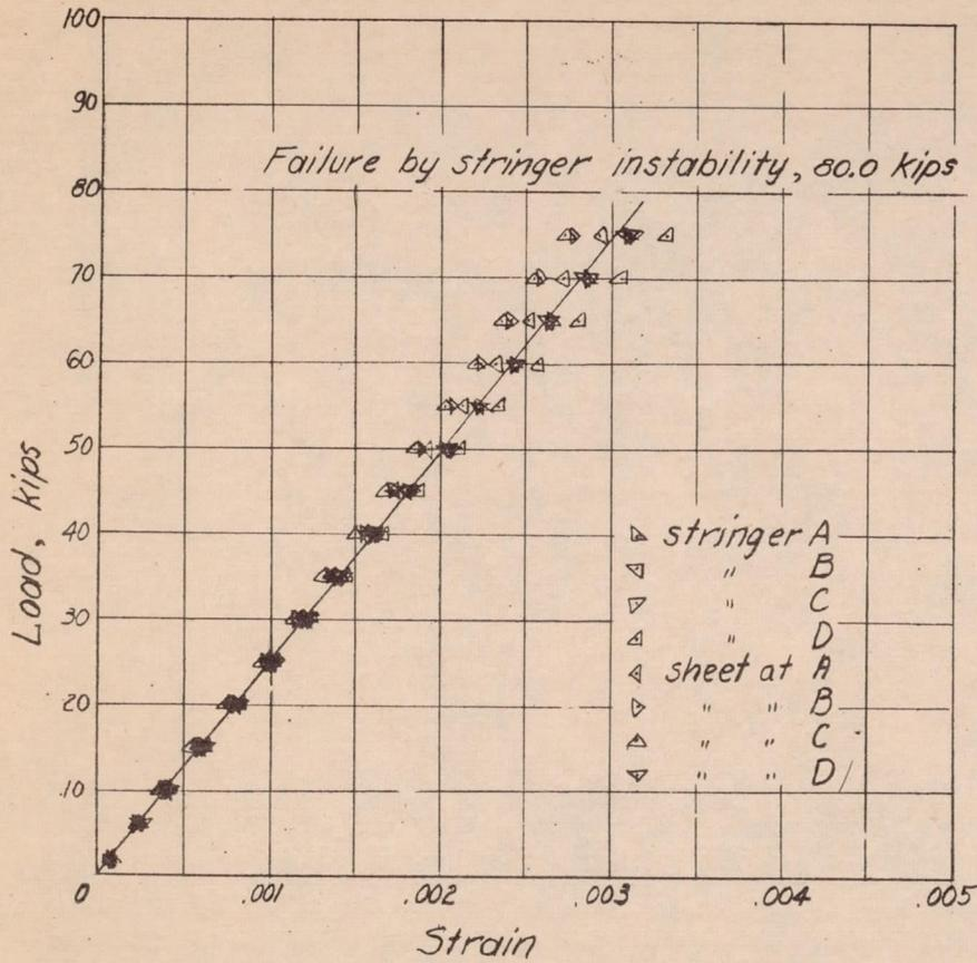
Figure 20.- Test of panel 15; radius, 25.5 inches.
