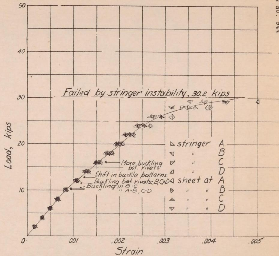
Figure 11.- Test of panel 6; radius, 19.1 inches.
