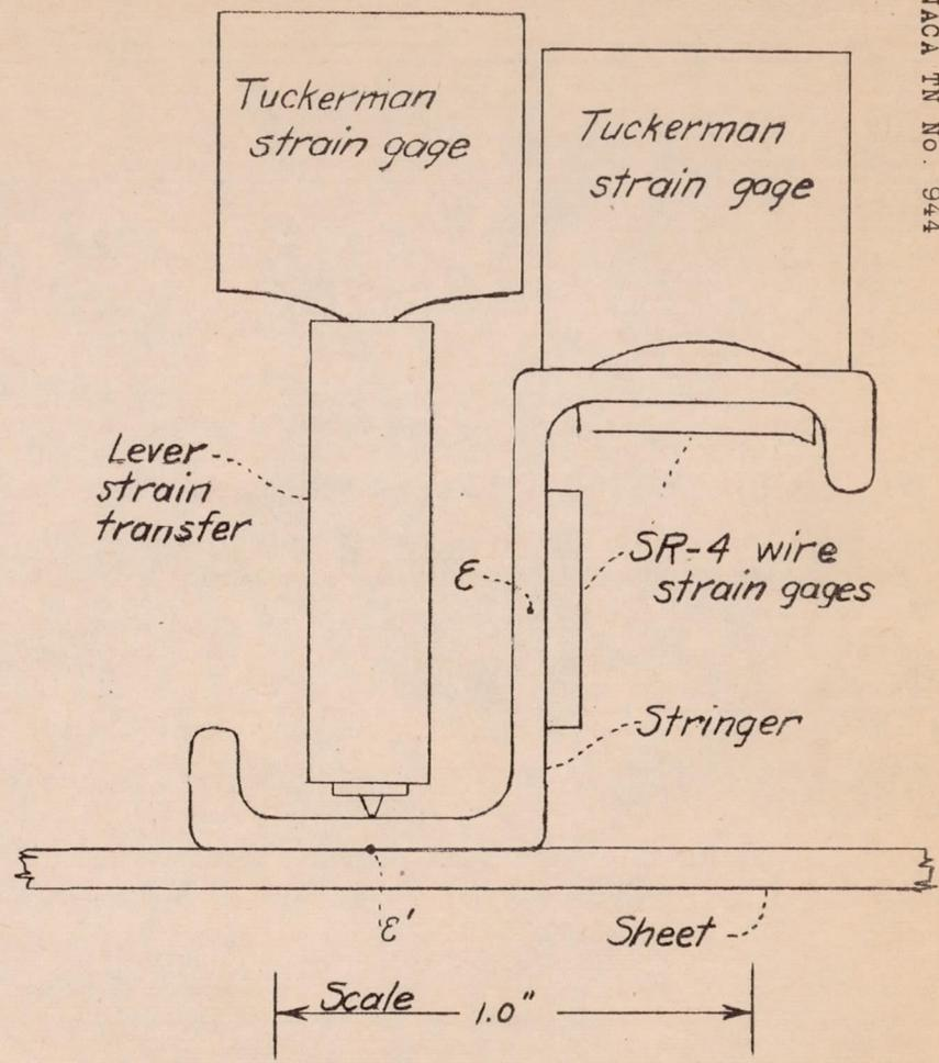
Figure 5.- Location of strain gages on stringer cross-section.
