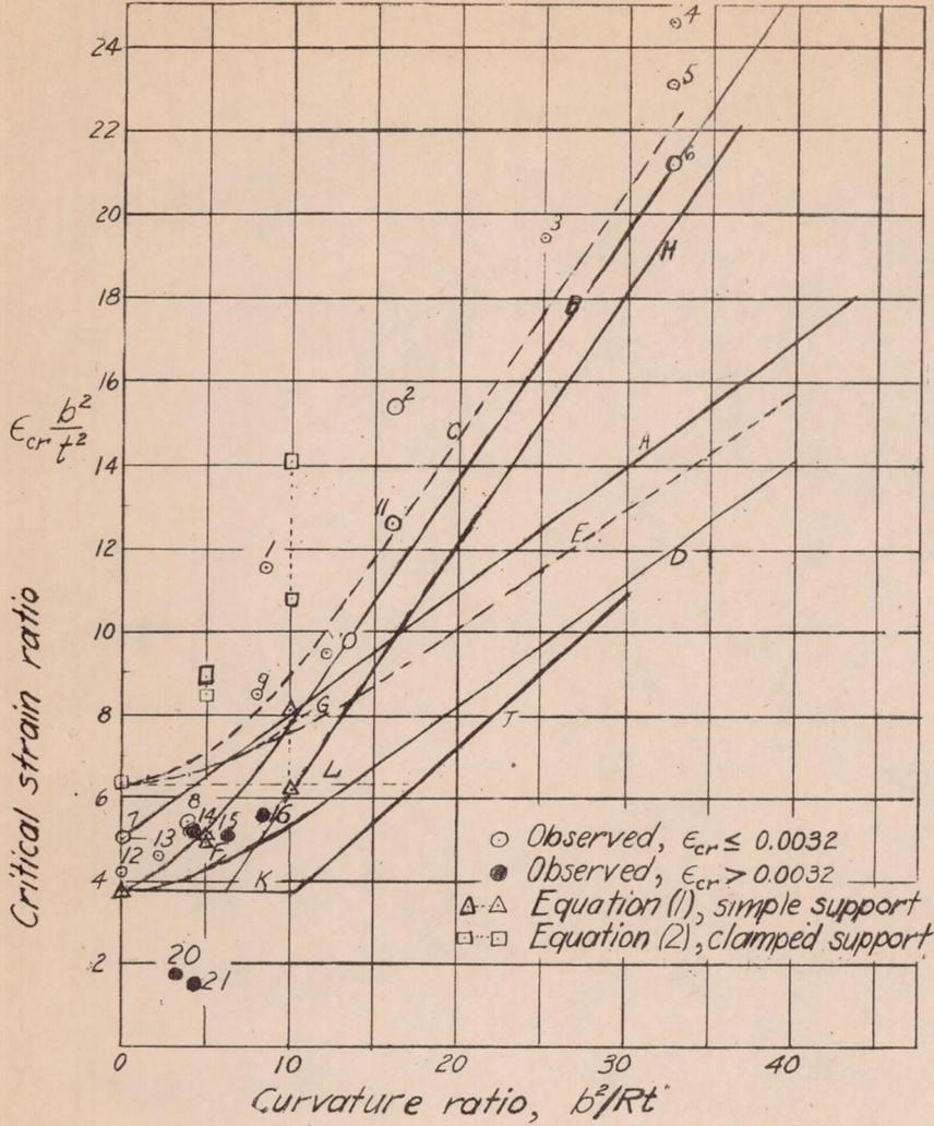
Figure 30.- Critical strain for buckling of curved sheet between stringers;  $b$  = stringer spacing;  $t$  = sheet thickness;  $R$  = radius of curvature;  $\epsilon_{cr}$  = strain for buckling between stringers.
