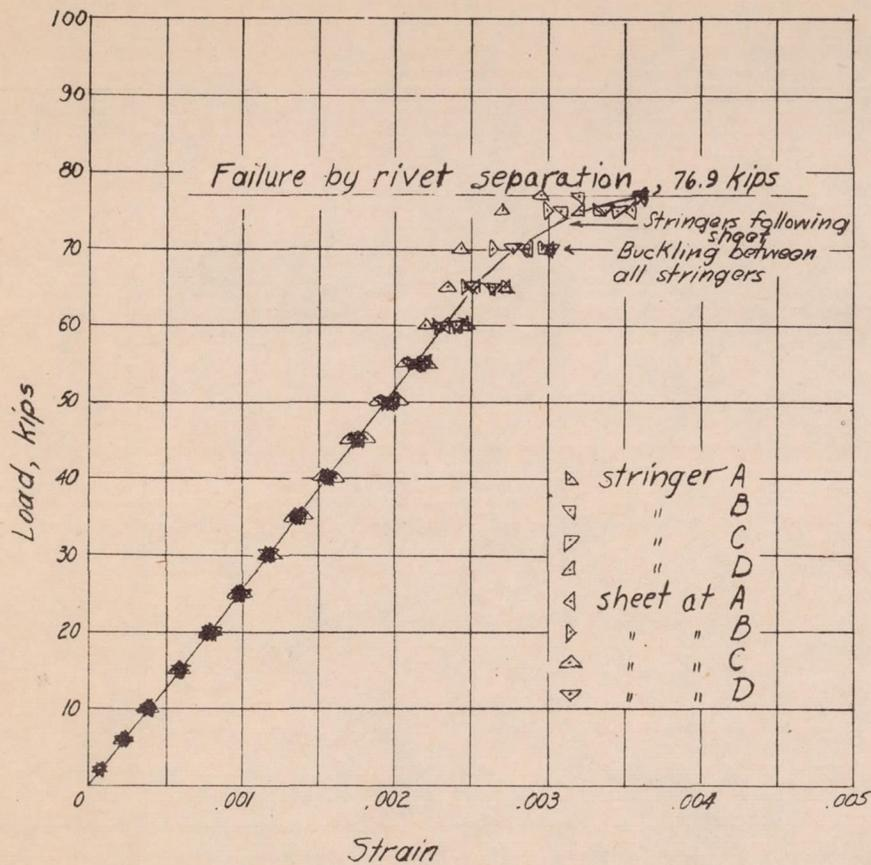
Figure 18.- Test of panel 13; radius, 76.5 inches.
