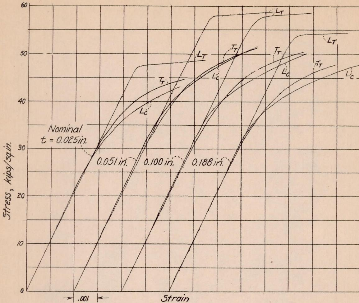
Figure 2.- Stress-strain curves of 24S-T aluminum alloy sheet used in panels.  $L_T$ , tension in direction of rolling;  $L_C$ , compression in direction of rolling;  $T_T$ , tension transverse to direction of rolling.
