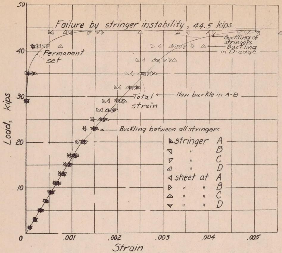
Figure 14.- Test of panel 9; radius, 38.2 inches.
