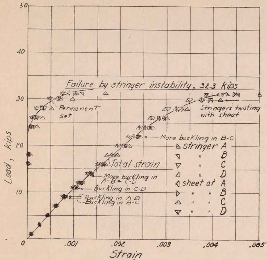
Figure 8.- Test of panel 3; radius, 25.5 inches.
