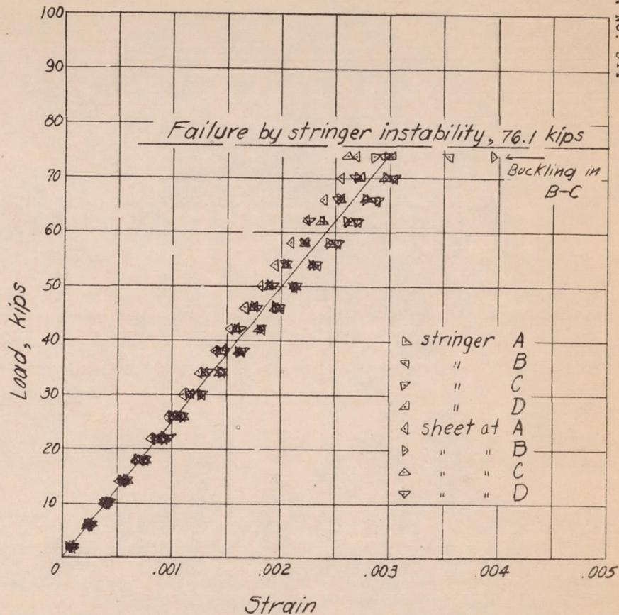
Figure 19.- Test of panel 14; radius, 36.5 inches.
