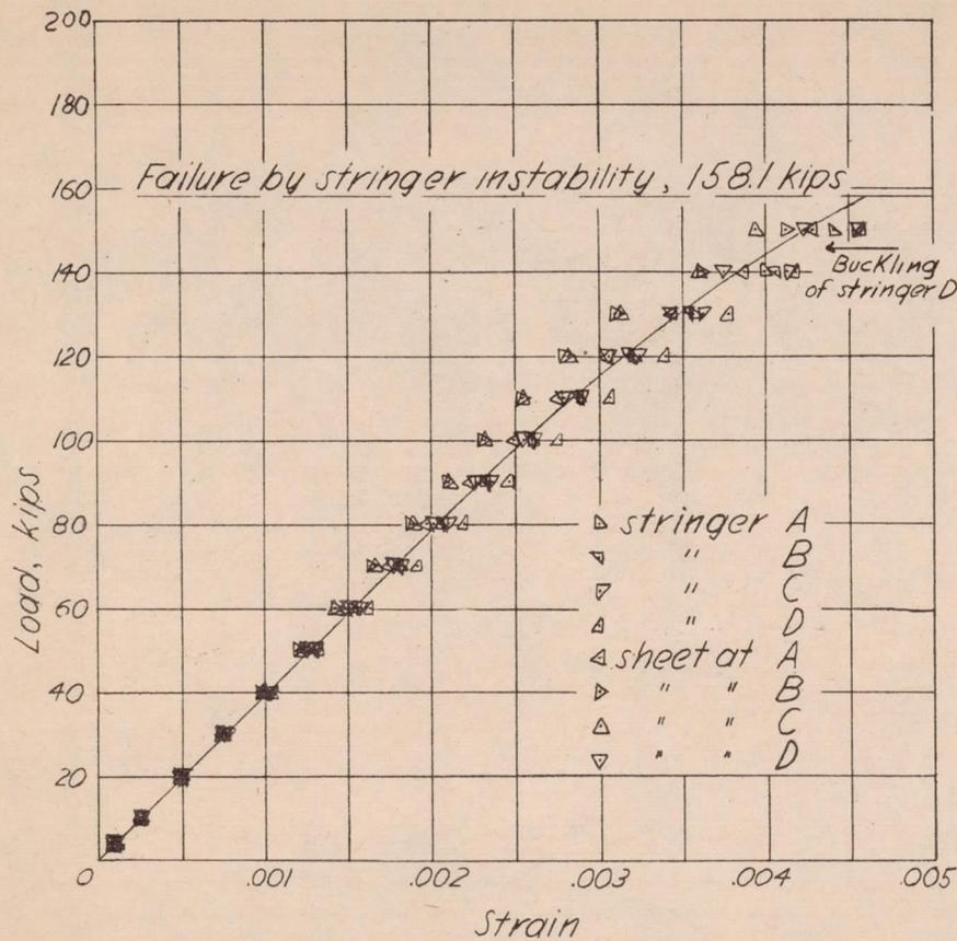
Figure 26.- Test of panel 21; radius 19.1 inches.
