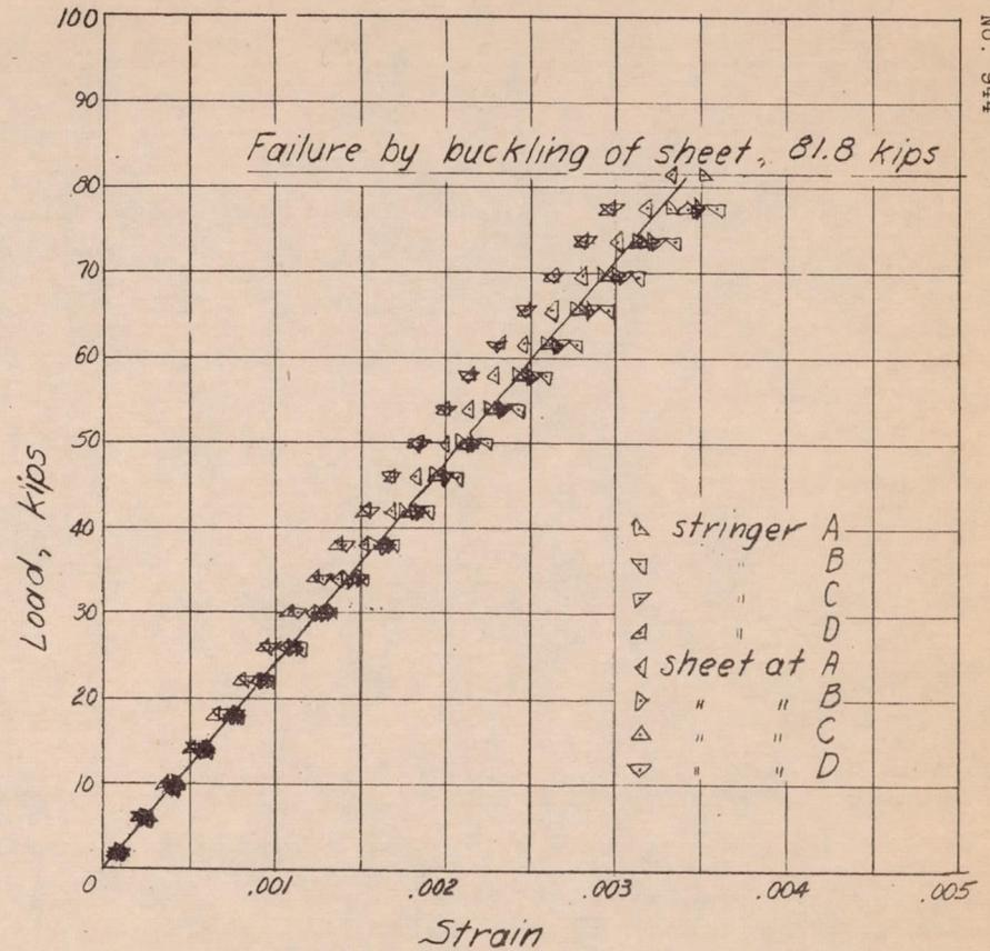
Figure 21.- Test of panel 16; radius, 19.1 inches.
