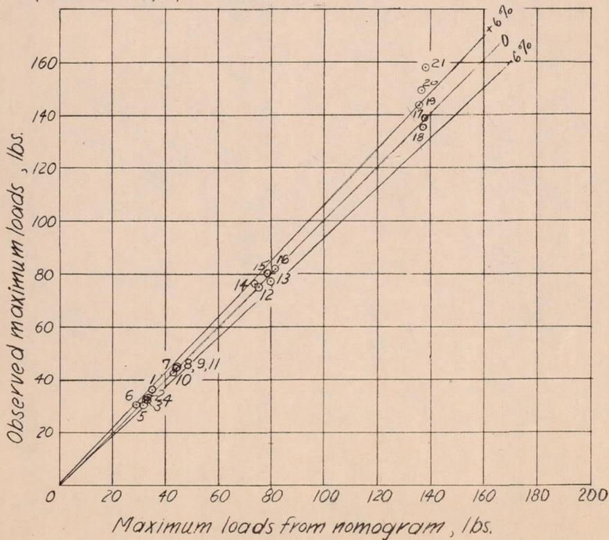
Figure 37.- Measured maximum loads against loads given by nomogram (figure 56 of reference 4).
