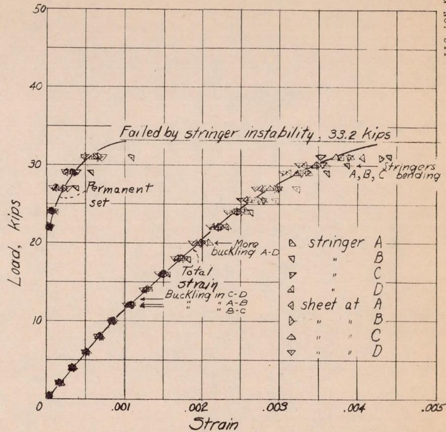
Figure 9.- Test of panel 4; radius, 19.1 inches.
