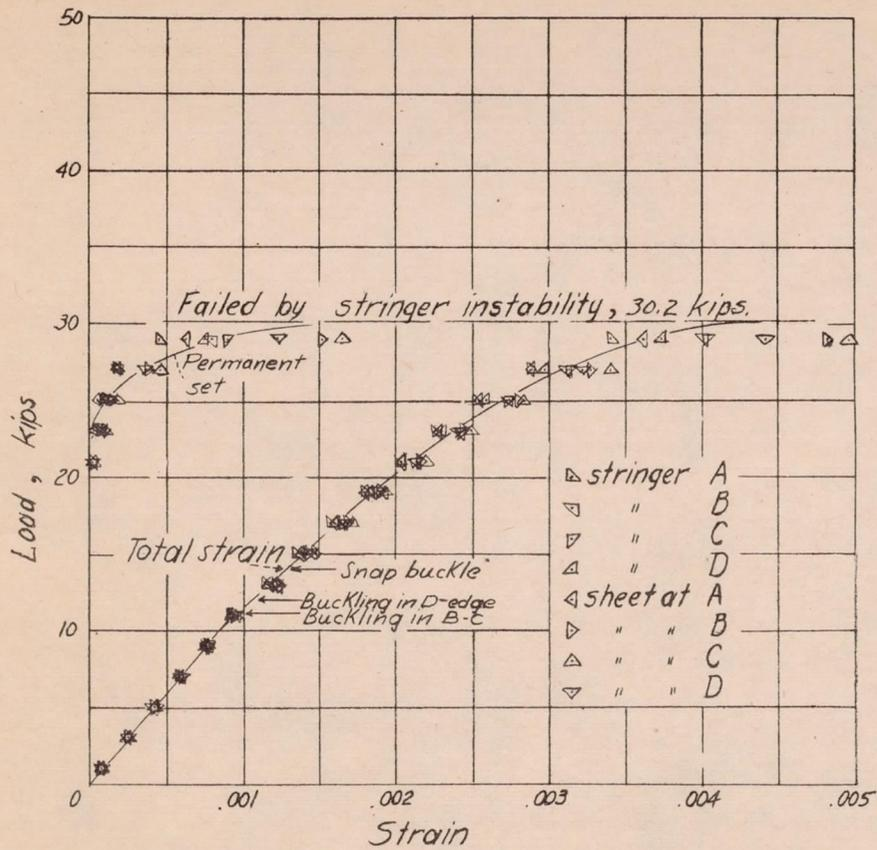
Figure 10.- Test of panel 5; radius, 19.1 inches.
