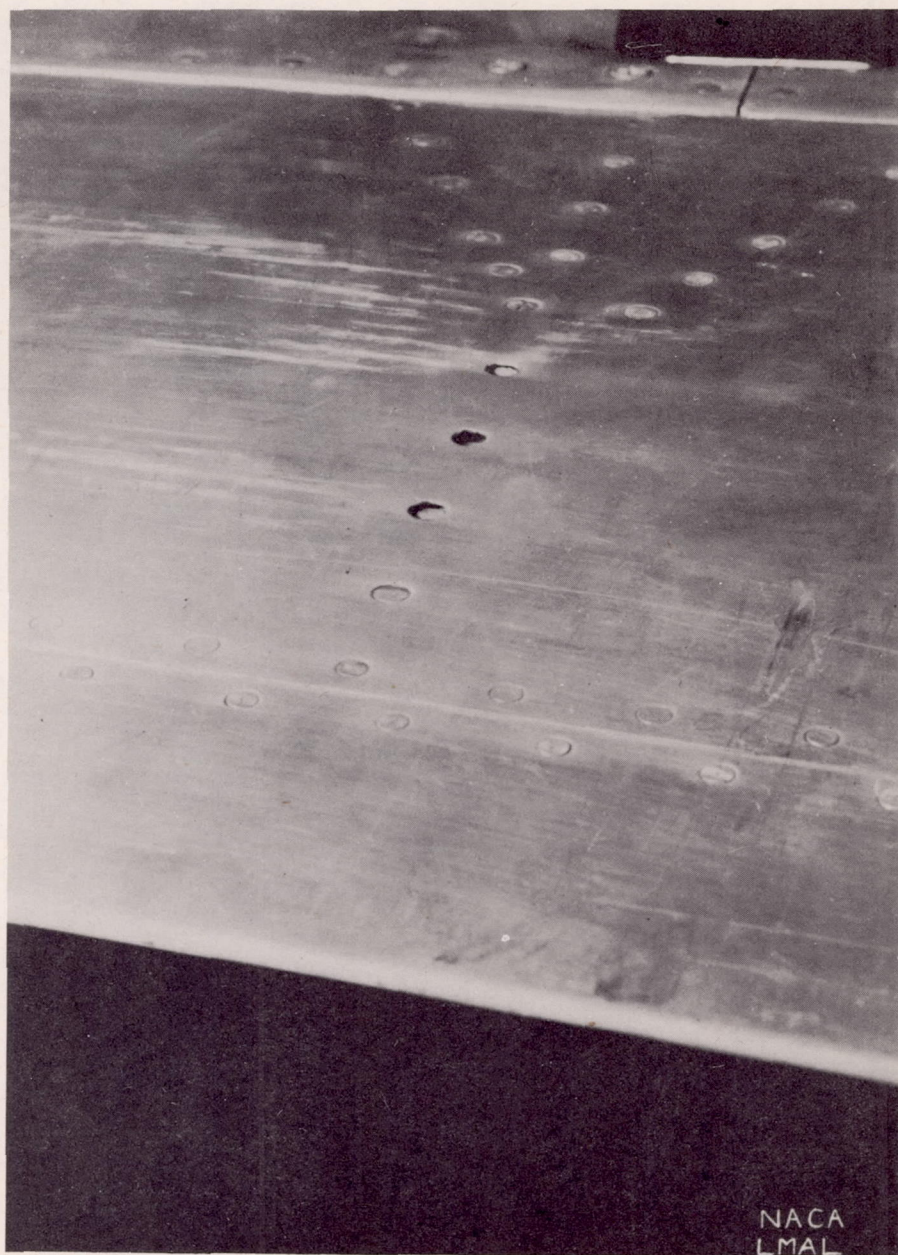
Figure 29.- Detail of upper-surface skin failure at station 50.
