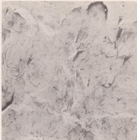
Figure 19. - Electron micrograph of running face of new nitrided-ring showing unworked surface area. Etched in potassium hydroxide. X10,000
