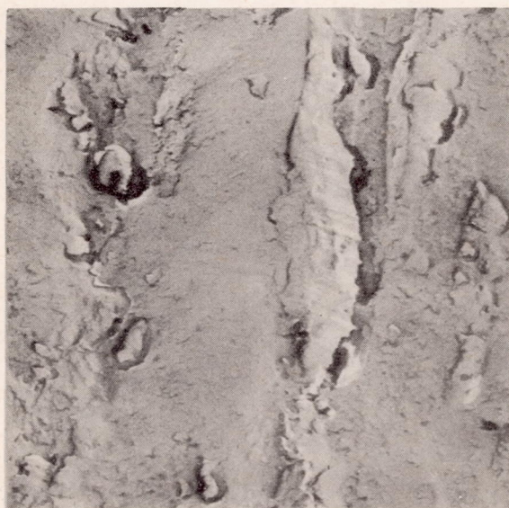
Figure 14. - Electron micrograph of cross section of used nitrided-steel piston ring showing nitrided case below worked-crystal area. Etched in nital. X10,000.
