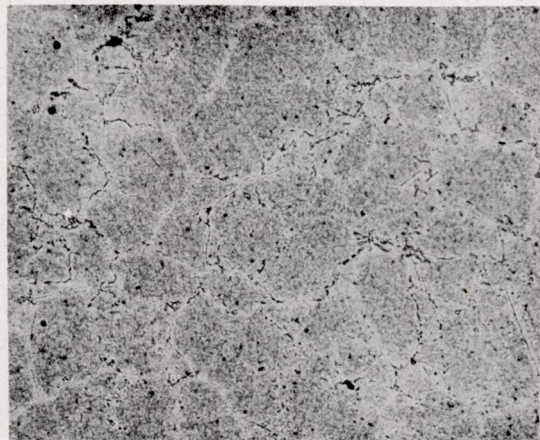
Specimen 1B4 - 2015 hours at 1350° F and 12,000 psi.
