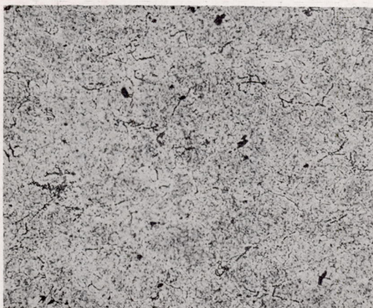
Specimen 2J4 - 2015 hours at 1350° F and 12,000 psi.
