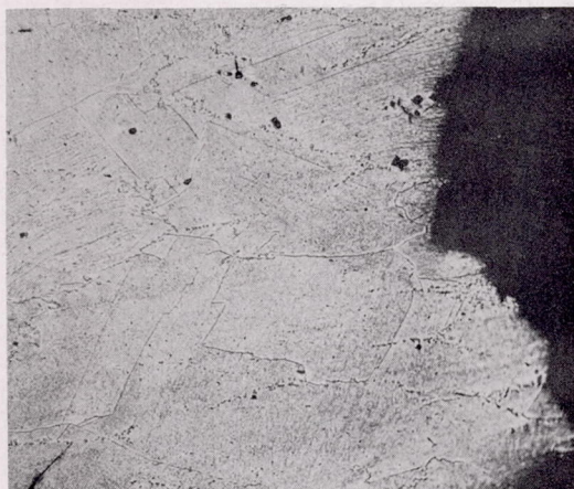
Specimen 2D4 - 1058 hours for rupture at 1200° F and 35,000 psi.
