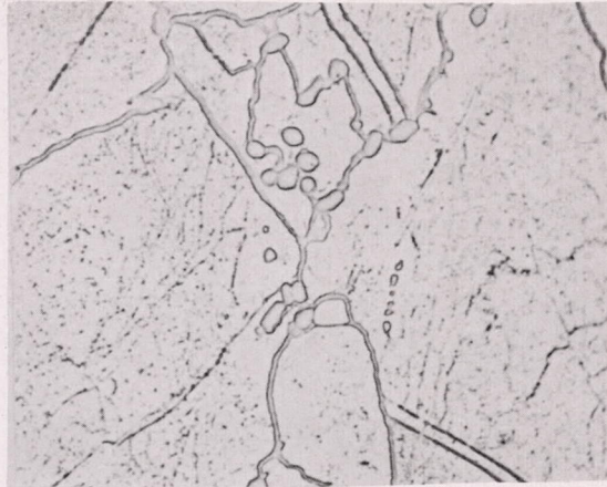
100X Specimen 1C5 - 613 hours for rupture at 1200° F and 40,000 psi.
