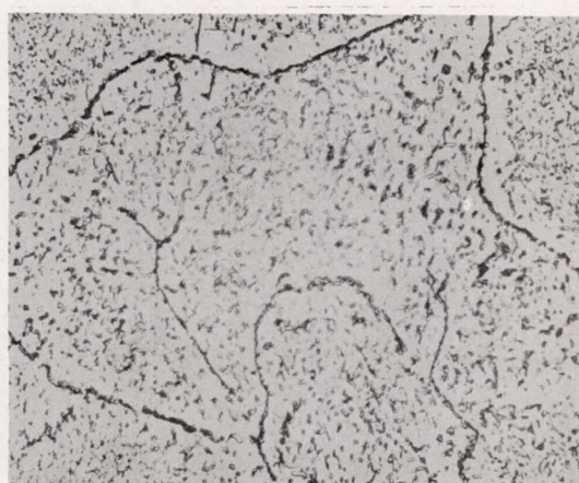
Specimen 2J4 - 2015 hours at 1350° F and 12,000 psi.
