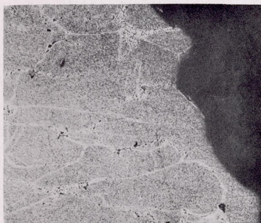
Specimen 2C4-2 - 729 hours for rupture at 1350° F and 21,500 psi.
