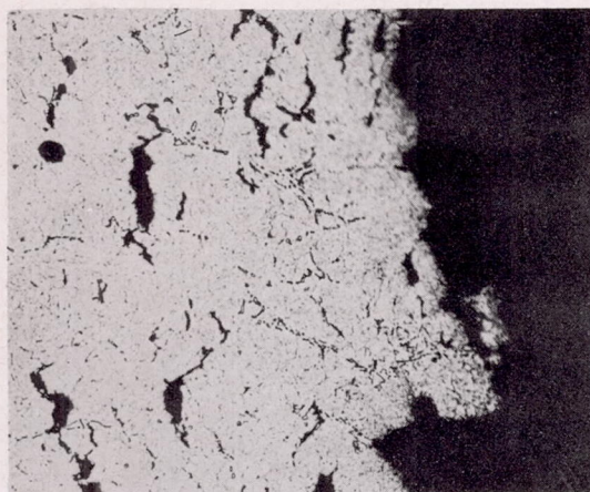
100X Specimen 1E4 - 449 hours for rupture at 1500° F and 14,000 psi.
