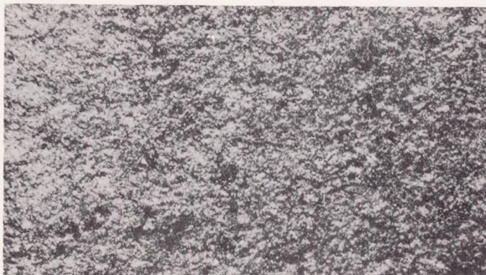
(c) 30X magnified view of coating L-2A (see fig. 10) which withstood treatment with little or no formation of tubercles. This photomicrograph should be contrasted with figure 11c, which is a magnified view of coating A-305 (see fig. 10) after formation of tubercles.
