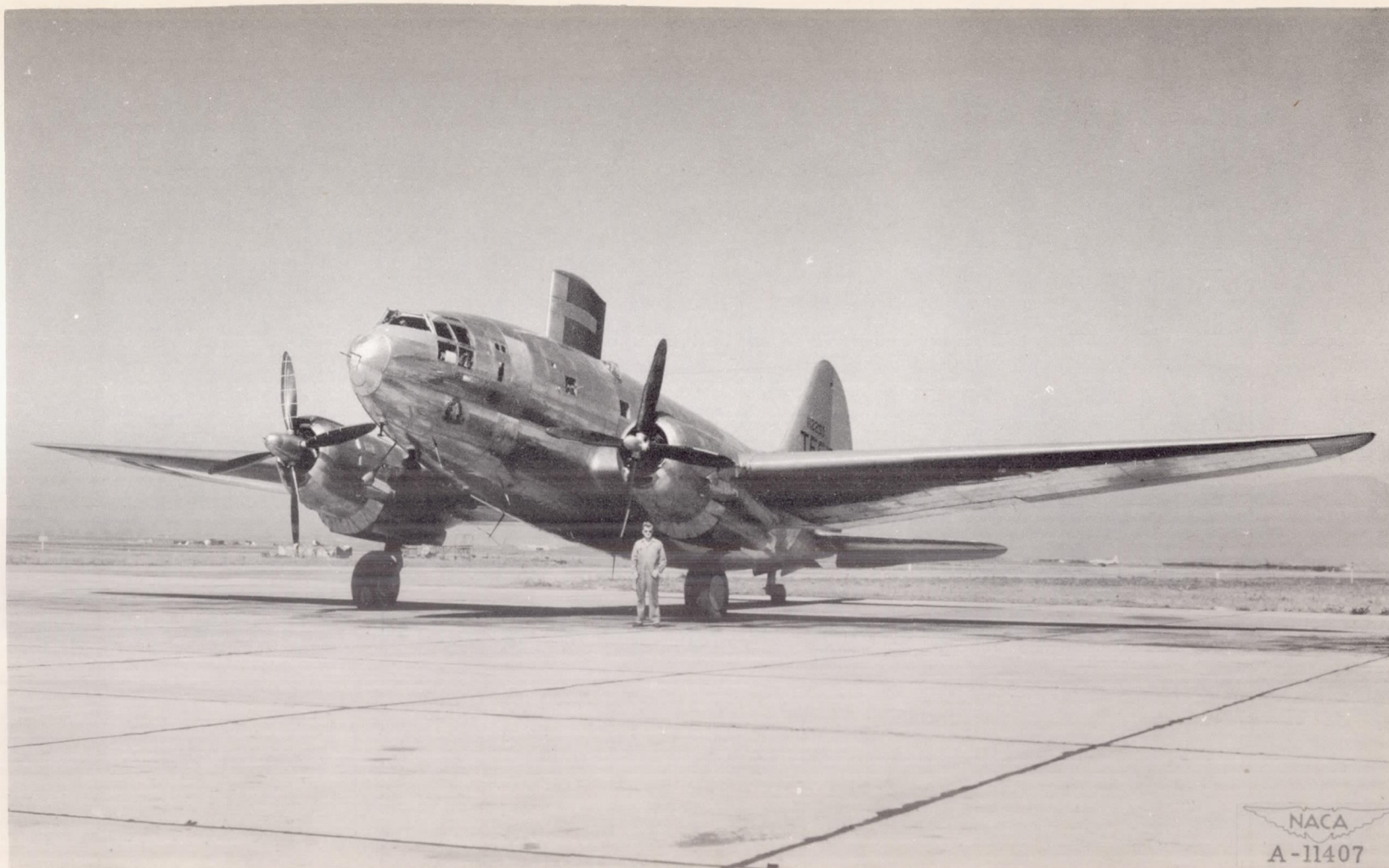
Figure 5.- C-46 test airplane as flown during the winter of 1946-47 showing the position of the airfoil models mounted on the fuselage.
