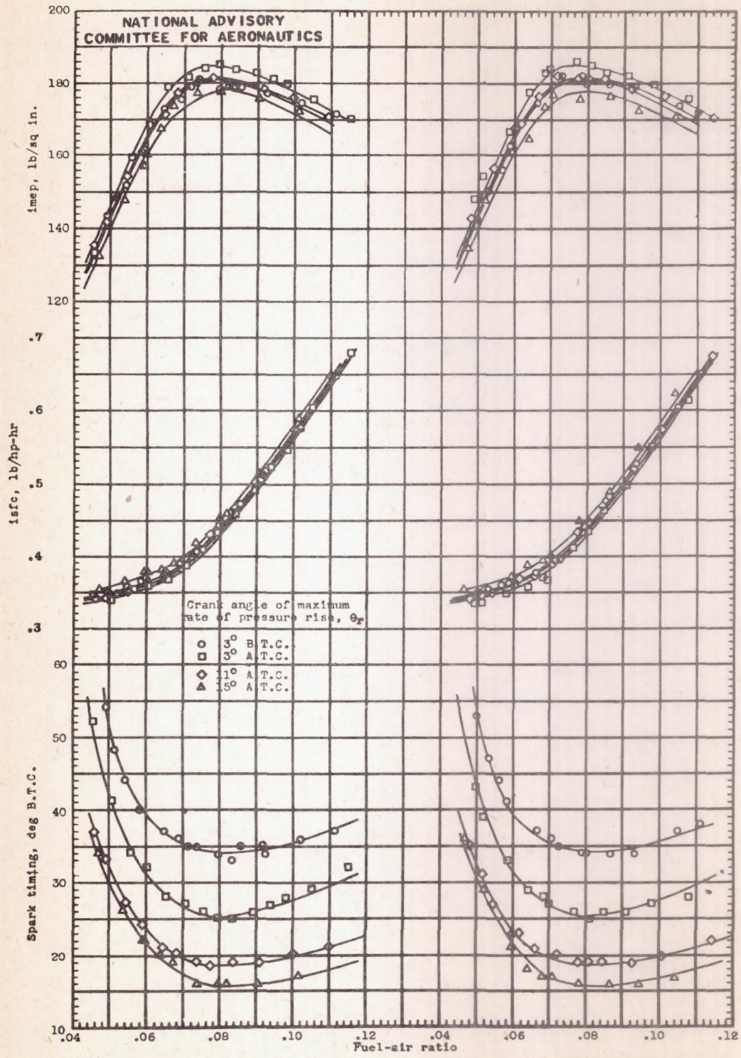
Figure 1. - Comparison of engine performance with spark timing manually controlled to maintain constant crank angle of maximum rate of pressure rise \theta_r and with spark timing automatically controlled to maintain constant crank angle of passage of flame front at ionization gap. (Paired curves in figs. 1(a) and (b) are the same. Runs of fig. 1(b) were conducted with automatic spark-timing control set to give same spark timing at fuel-air ratio of 0.085 as was obtained in runs of fig. 1(a).)
