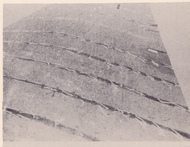
Figure 10.- Flow conditions over upper surface of airplane wing as indicated by wool tufts. Airplane lift coefficient, 0.2.
