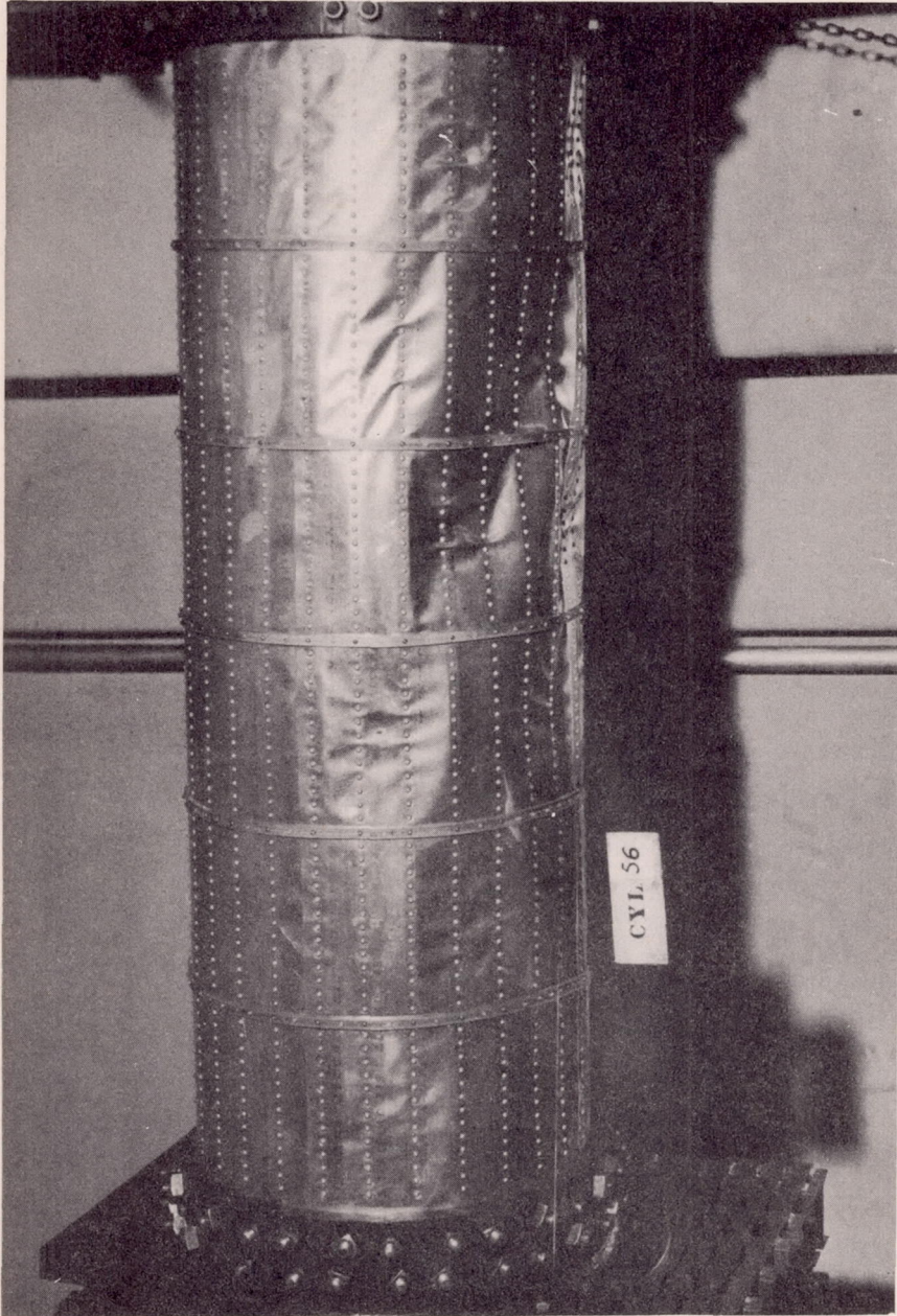
Figure 35.- Photograph of cylinder 56 after buckling.
