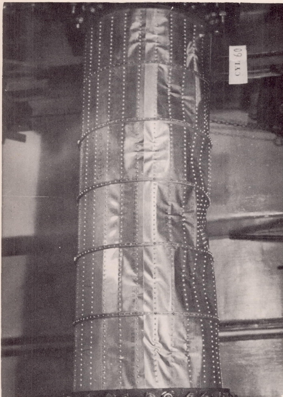
Figure 39.- Photograph of cylinder 60 after buckling.
