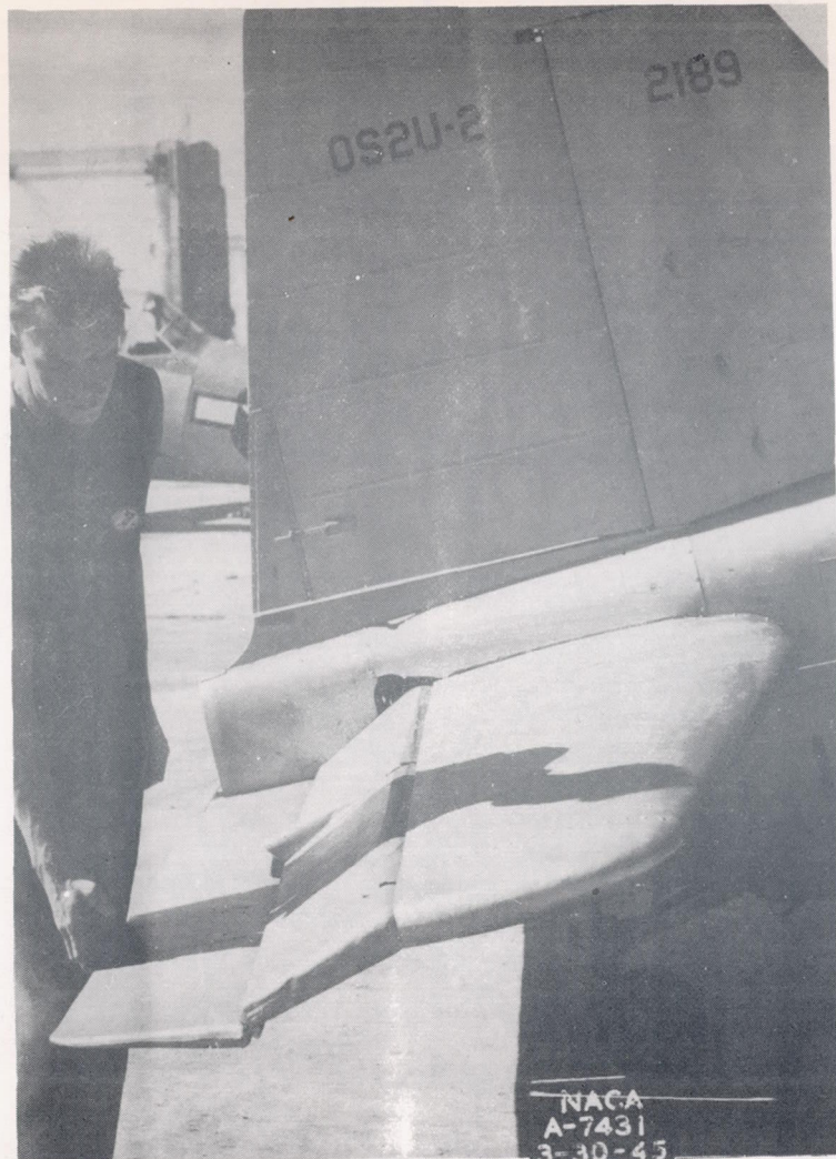
(a) Trimmer full down, elevator full up. (b) Trimmer full down, elevator full down. Figure 3.- Side view of the double-hinged horizontal-tail surface, trimmer and elevator deflected.
